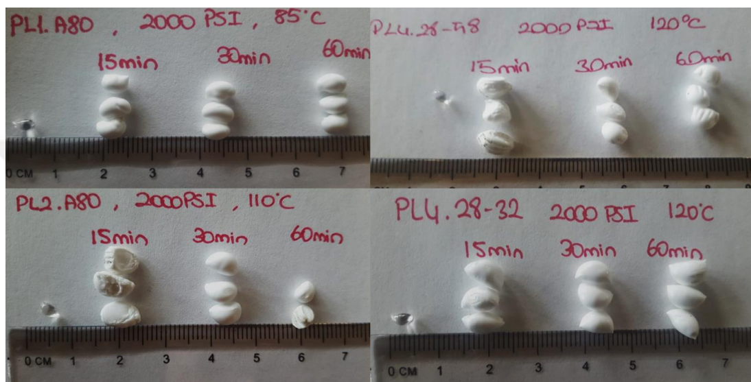
Figure 4.20: Foams of TPUs at various saturation times.
