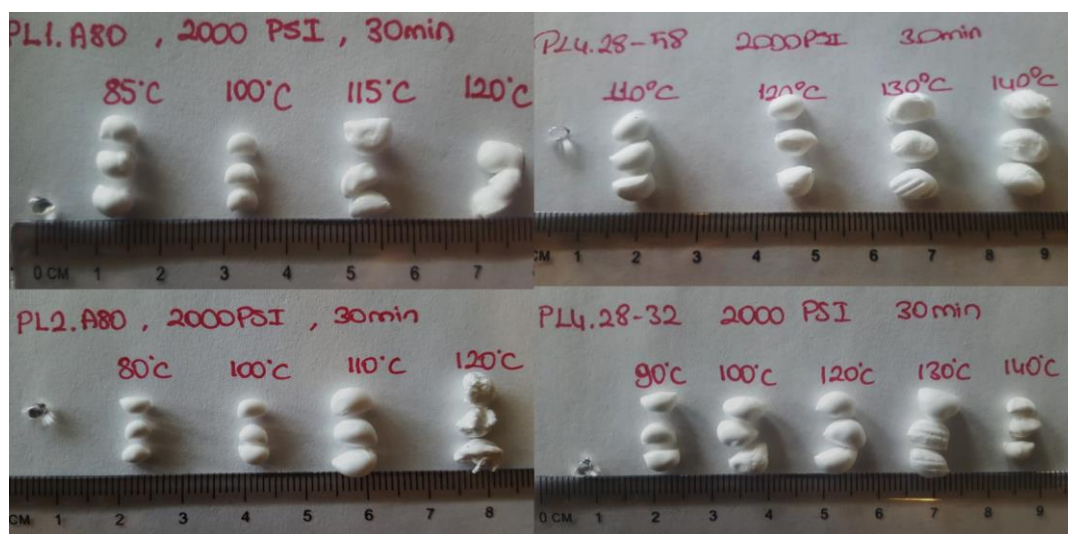
Figure 4.8: Foams of TPUs at various saturation temperatures.
