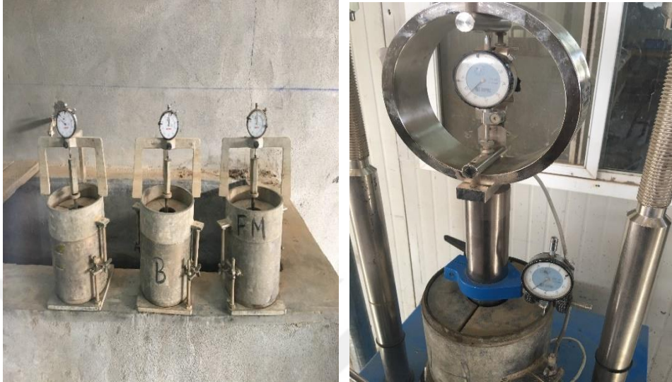
Figure 4.15. Picture of laboratory work CBR test.
