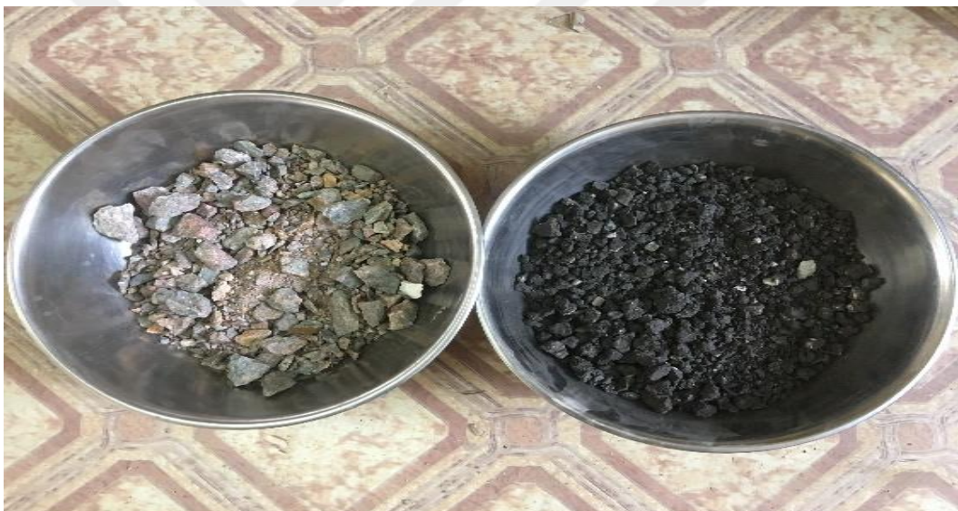
Figure 5.6. Blended RAP/Crushed gravel (0/31,5)
