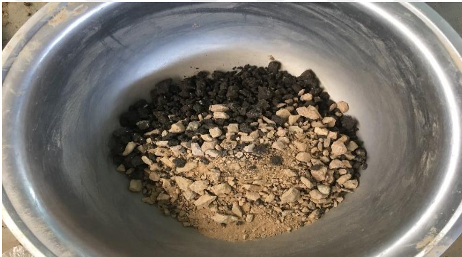
Figure 4.6. Blended lateritic soil with reclaimed material.
