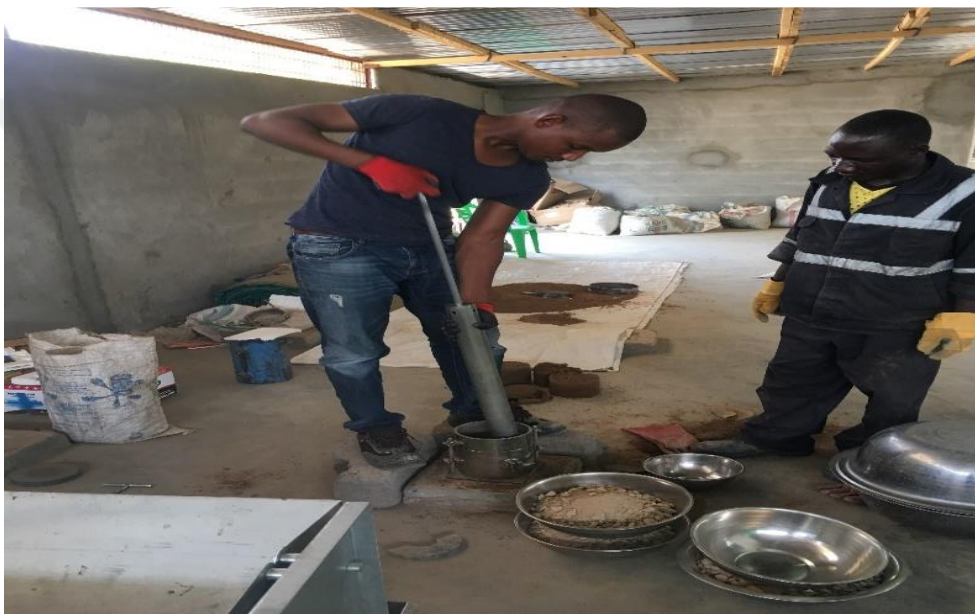
Figure 4.12. Picture of laboratory work Proctor test.
