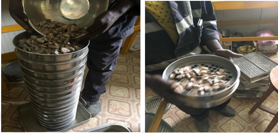
Figure 5.4. Crushed gravel particle size test pictures.
