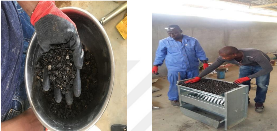
Figure 1.1. Reclaimed Asphalt Materials used in the Study
