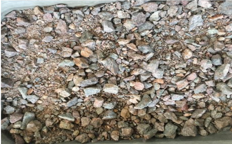
Figure 3.6. Crushed stone 0/31,5 mixture of aggregates
