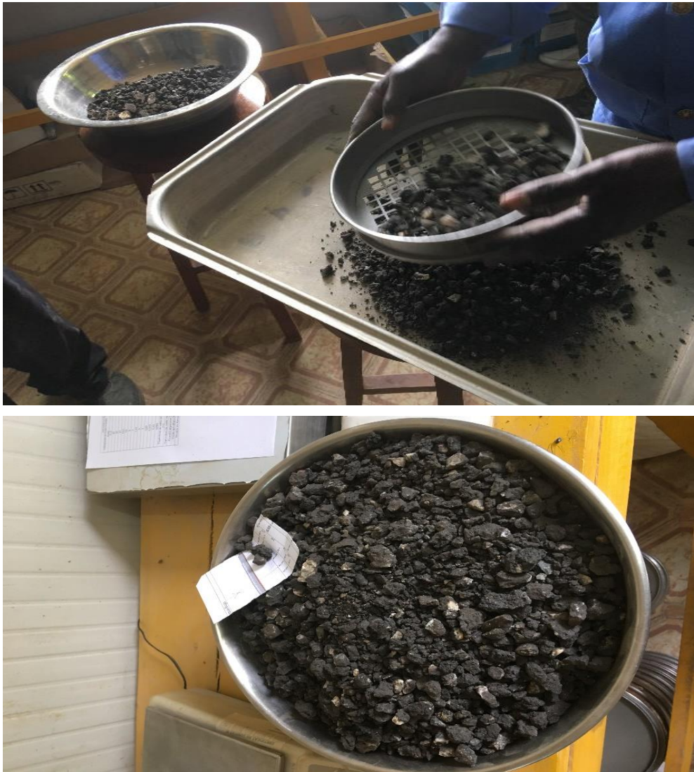
Figure 4.4. Reclaimed asphalt material Particle size test.
