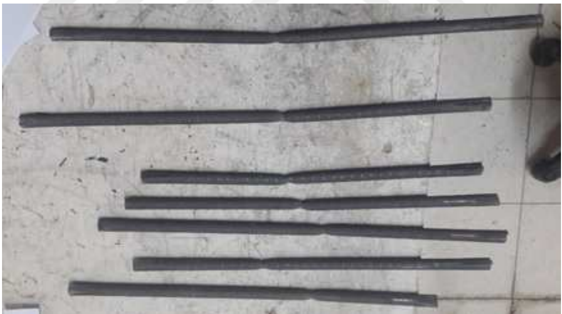
Figure 3.17: Configuration of the steel rebars after tensile test
