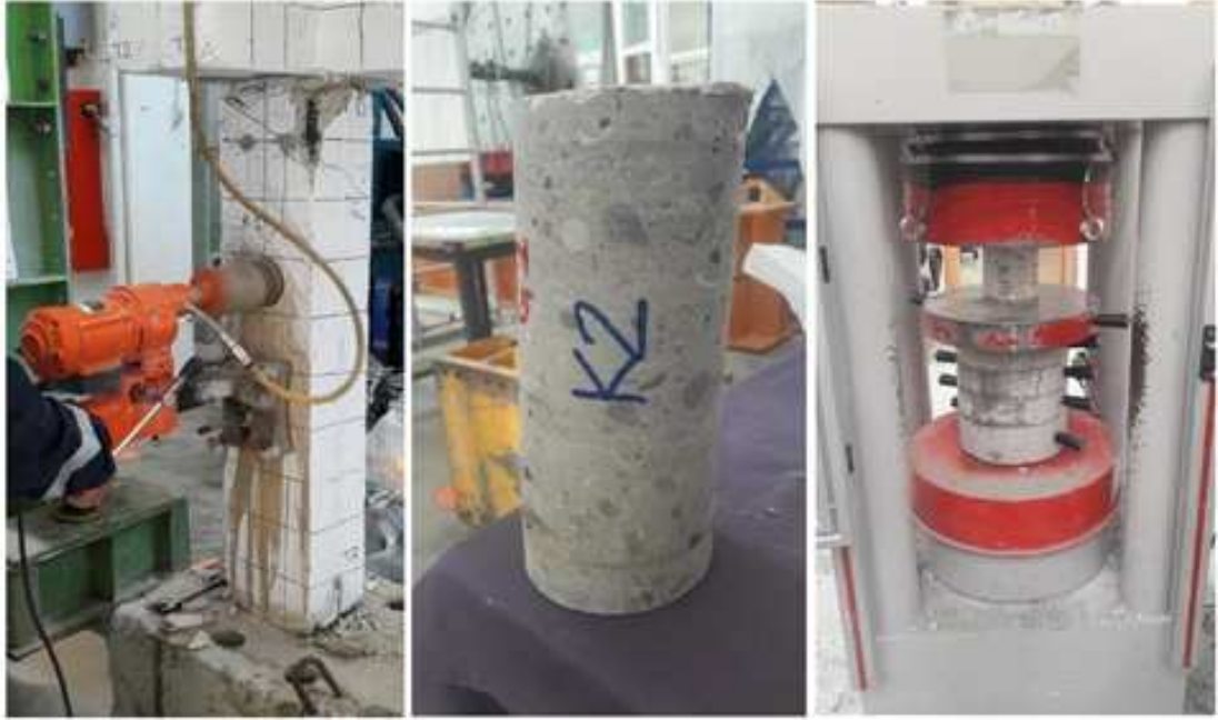
Figure 3.12: Drilling and testing of core specimens
