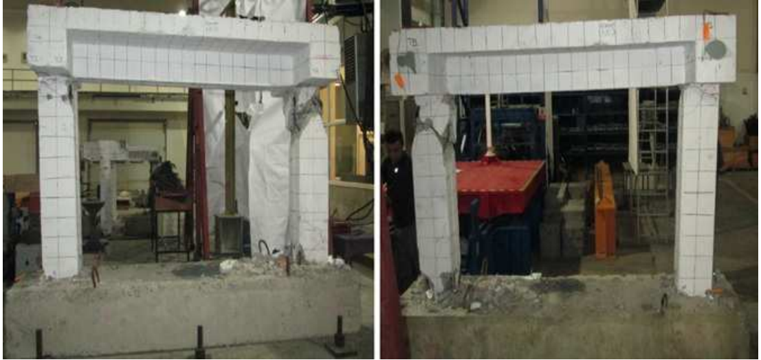
Figure 4.6: Front view and back view of the specimen-A, respectively, at the end of the test
