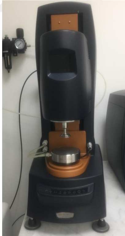
Şekil 3.2. Reometre (TA, Discovery HR-3 Hybrid Rheometer)
