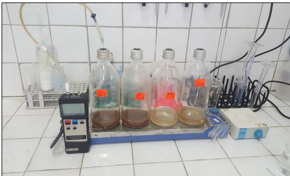
Figure 3.1 : Adaptation experiments for ET and DMS in 1200 mL bottle inoculated with 100 mL inoculum at VSS = 300 and 3000 mg/L.
