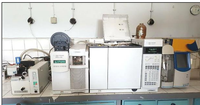
Figure 3.4 : Alignment GC-7090A and MSD for odorous compounds measurements.
