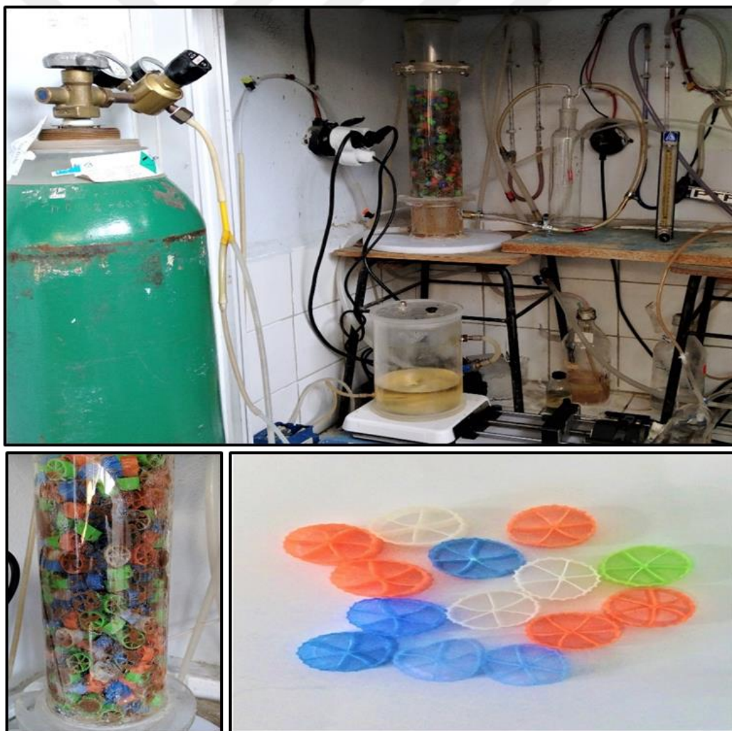
Figure 3.5 : Real photos of the laboratory-scale of ABTF model and packing medium.
