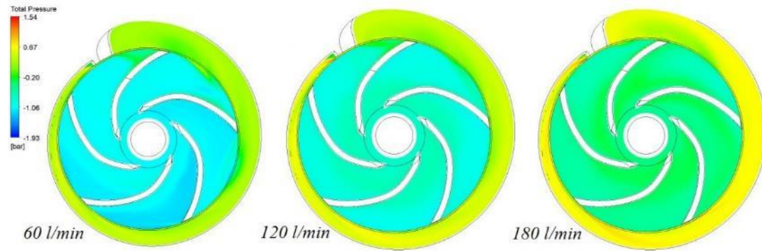
Figure 3.34. Total pressure distribution on the mid-section of Pump-3 (bar)
