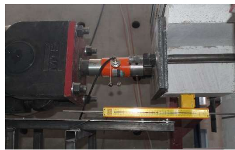
(b) Close view of MTS-frame connection
