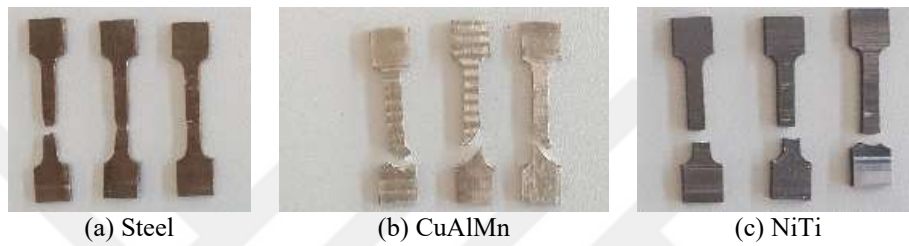
Figure 3.13. Tested dog-bone shaped specimens of upgrading materials
