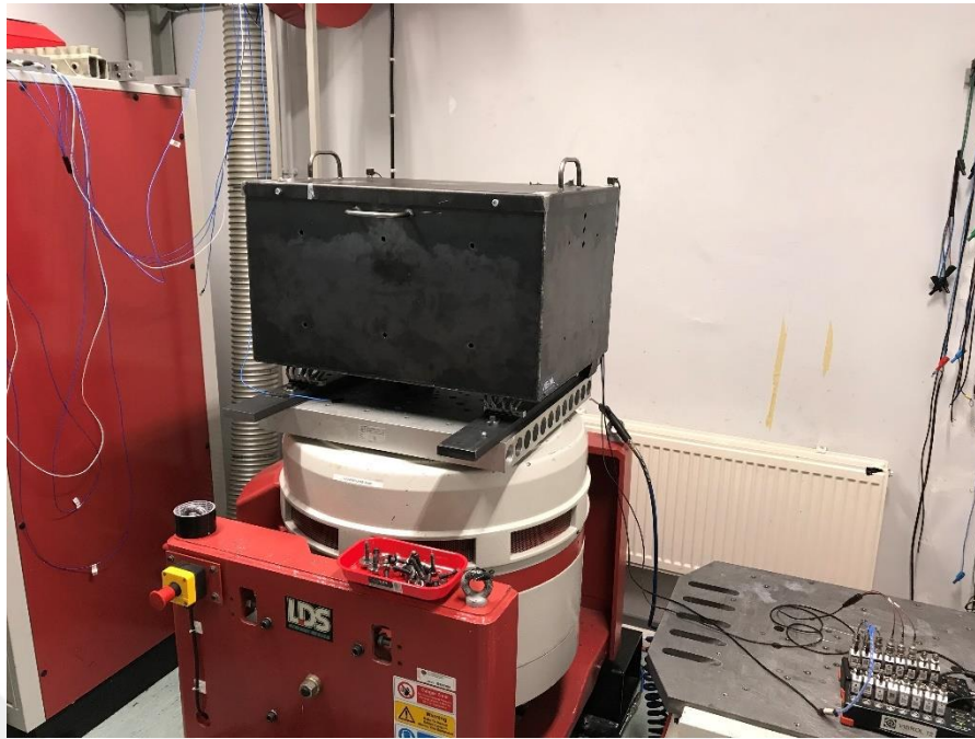
Figure 3-7 Electromagnetic Shaker Measurement of Electric Cabinet
