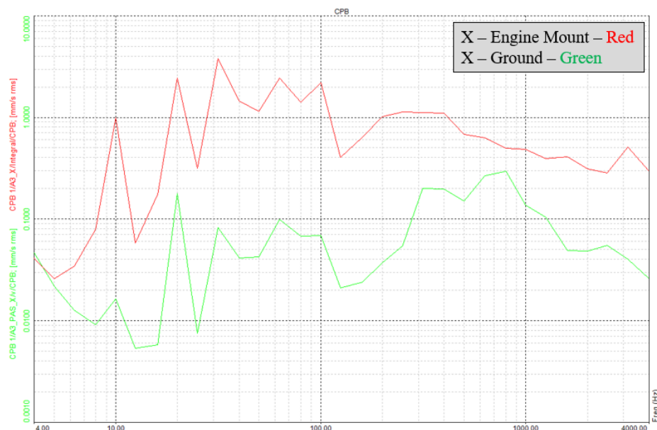
Figure 4-12 Structure Borne Noise Analysis (1/3 Octave Band Analysis) of Nominal Speed Measurement at Point A3 in Longitudinal Direction
