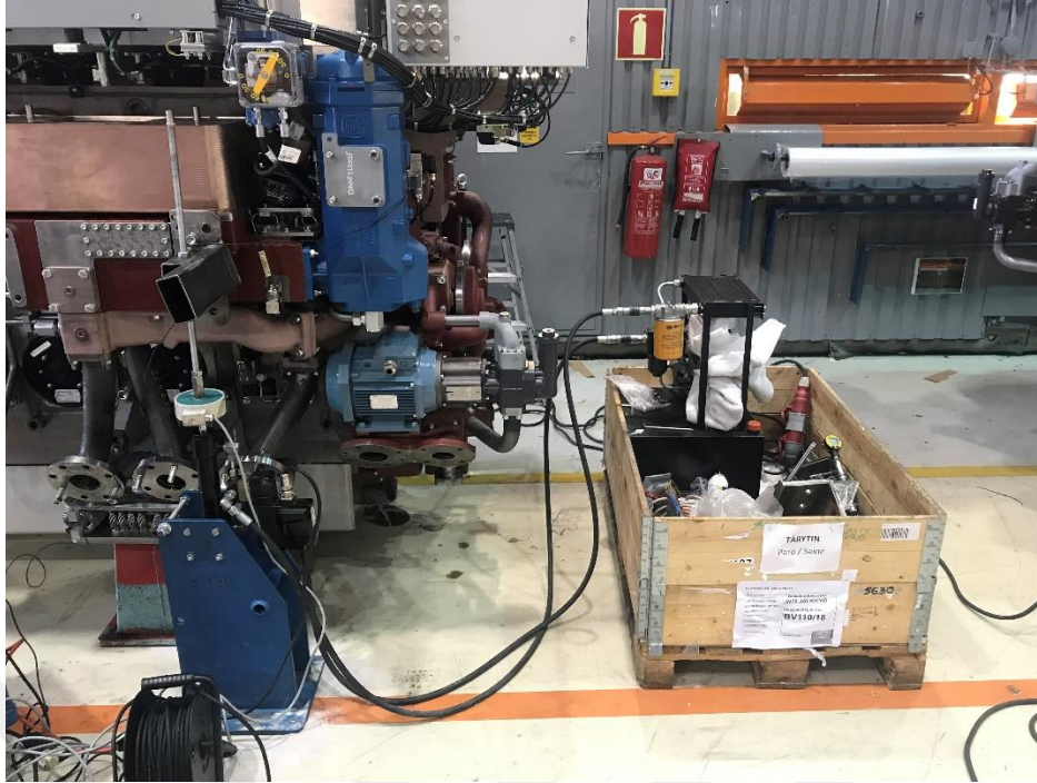
Figure 3-6 Hydraulic Shaker Measurement of the Engine
