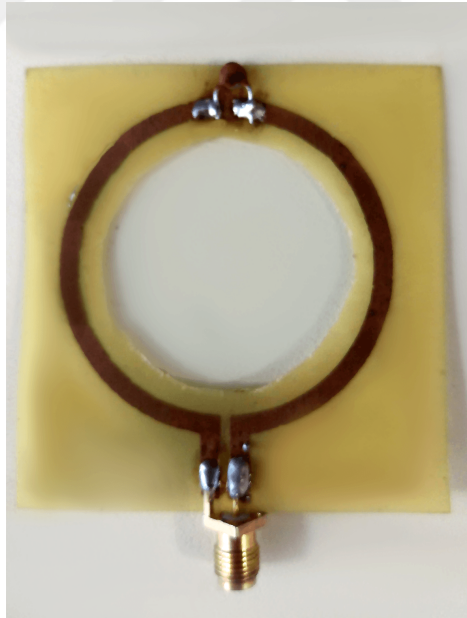
Figure 3.2. Photograph of an example antenna with C_{\text{tuning}} and SMA connector.
