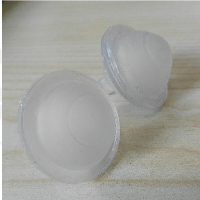
Figure 5.6. Photograph of the fabricated mechanical eyes from PDMS.
