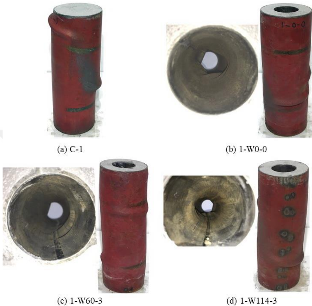
Figure 6.18 Failure modes of C-1, 1-W0-0, 1-W60-3 and 1-W114-3 specimens
