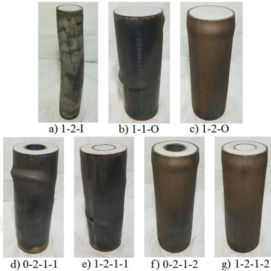
Figure 4.13 Failure modes of the specimens with normal strength concrete and thicker inner steel tube
