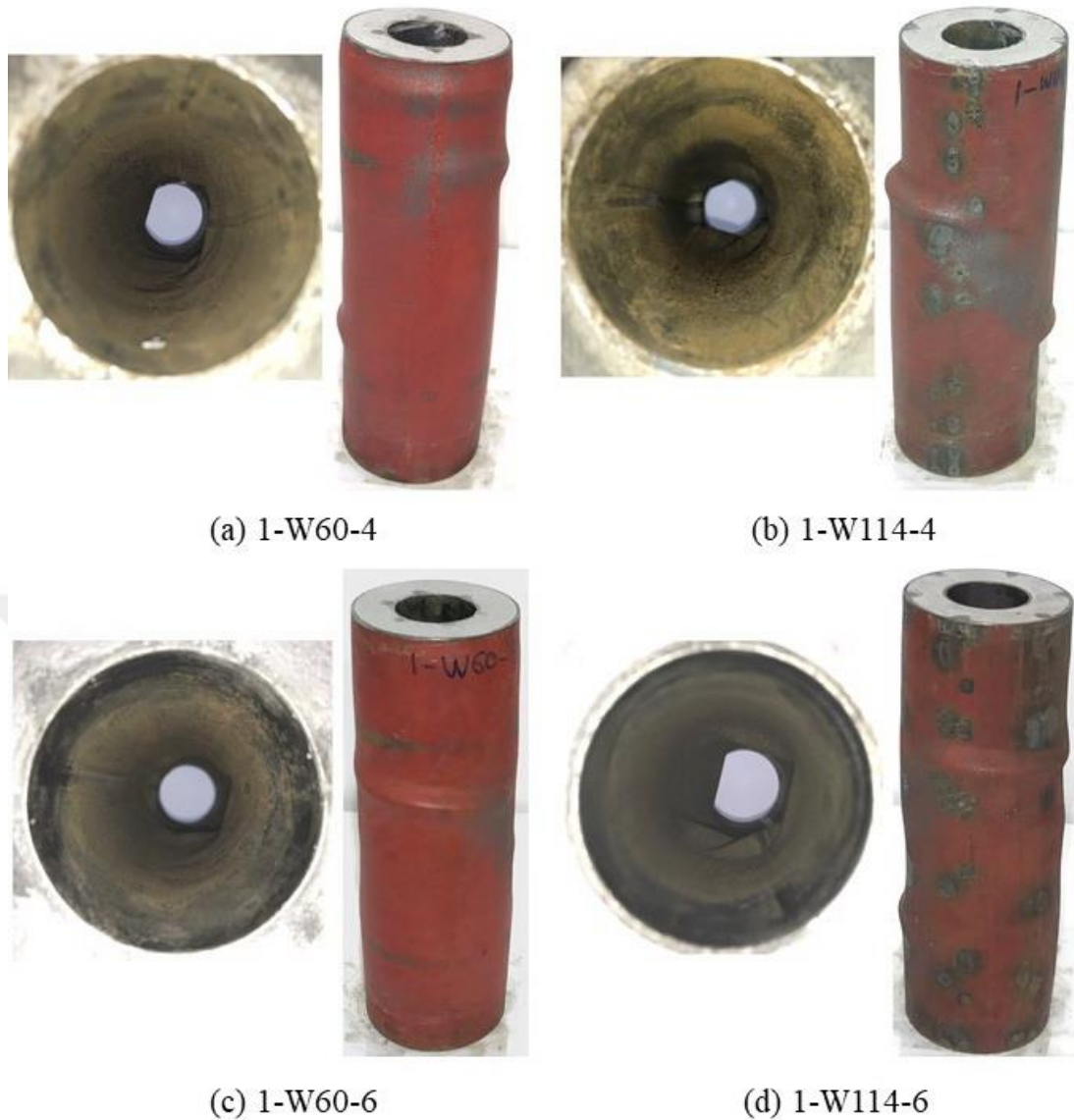
Figure 6.19 Failure modes of 1-W60-4, 1-W114-4, 1-W60-6 and 1-W114-6 specimens
