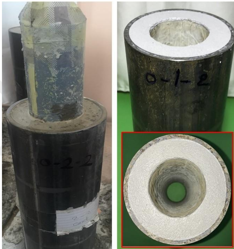
Figure 5.8 Manufacturing process of the specimen with hollow concrete
