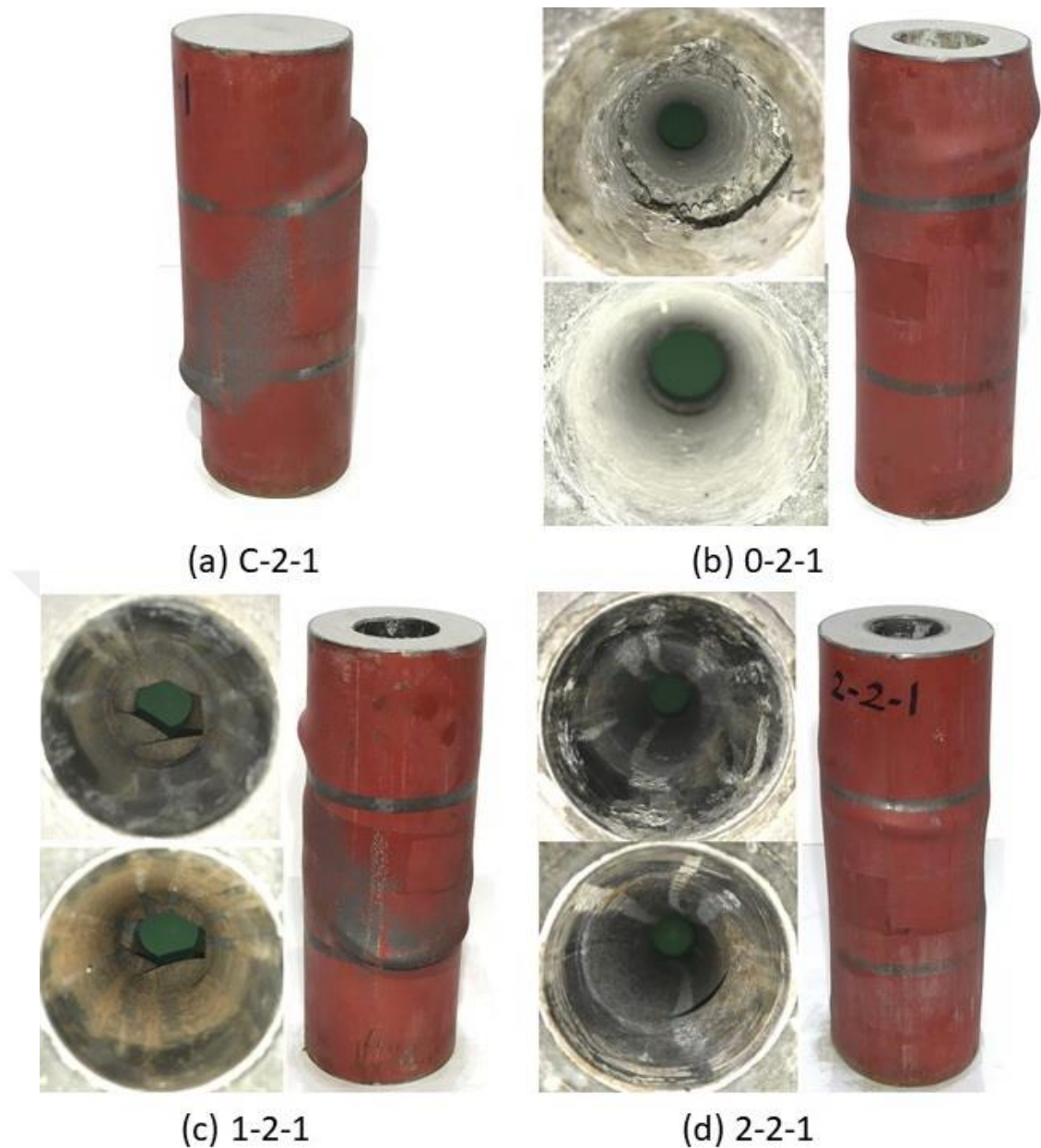
Figure 5.18 Failure modes of the columns in Set 4
