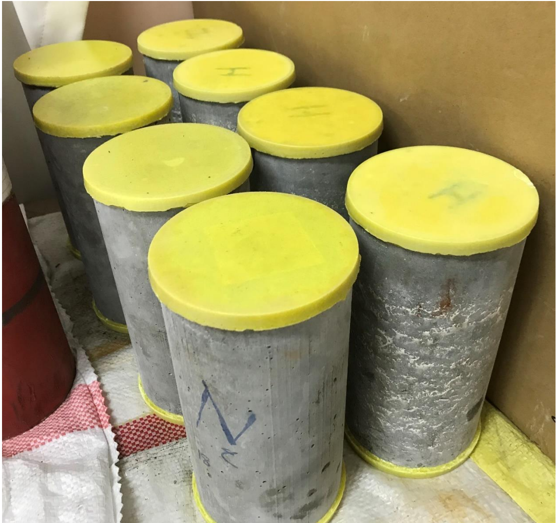
Figure 5.6 Cylinder concrete specimens
