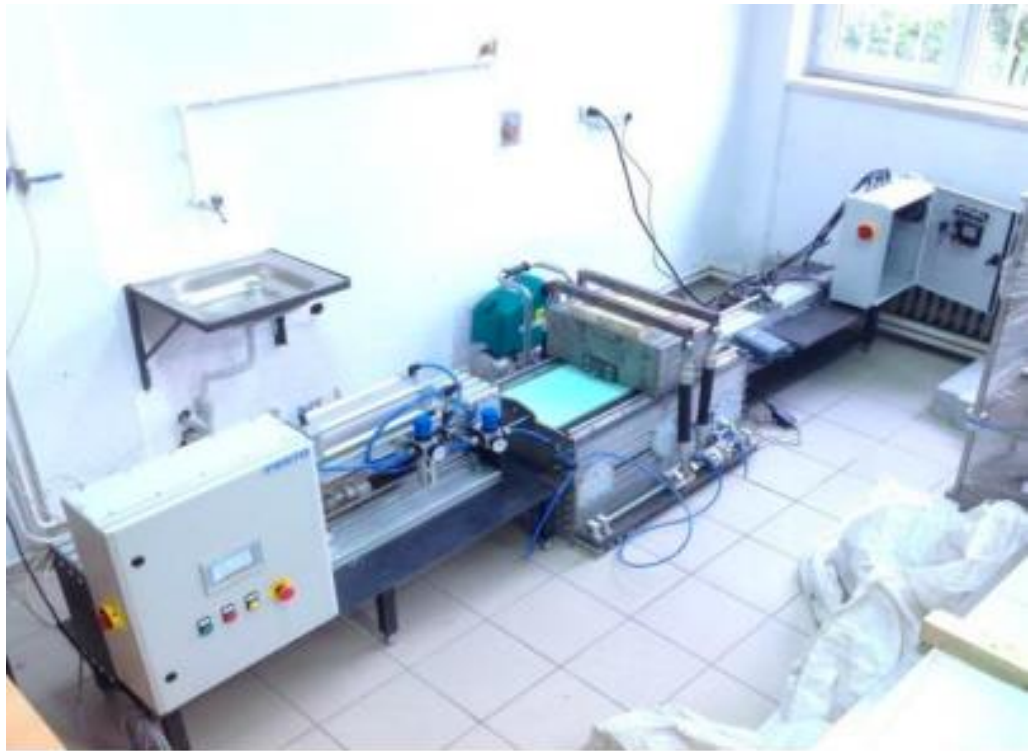
Figure 2.37. Large displacement constant contact area shear device [40].
