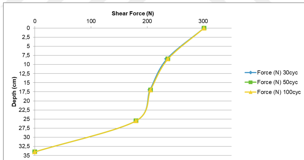
Figure 4.51. Shear of the Segmental Pile with Post-Tension Force 750 N in Loose Soil.
