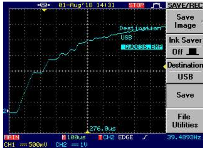
Figure 5.6 Charging capacitor waveform in loop filter during tuning process
