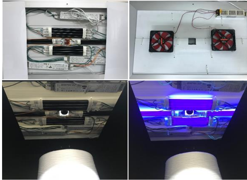
Figure 3.12 Machine vision system-Lighting unit
