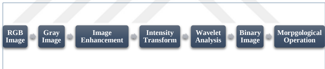
Figure 4.3 Flow chart of the Wavelet filter algorithm
