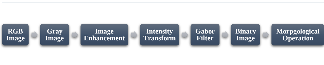
Figure 4.1 Flow chart of the Gabor filter algorithm
