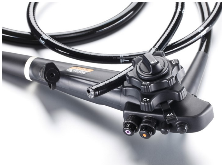
Figure 1.2. The distal end and the control knob of a colonoscope. Reprinted from [12].
