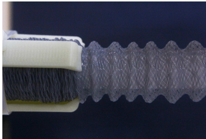
Figure 3.18. An image of the sheath reservoir and feed. Flexible sheath is released when its diameter is reduced to a certain value via axial force.
