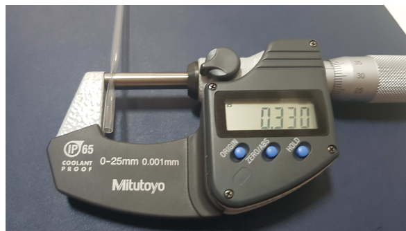
Figure 4.2. Thickness of the manufactured double layered tubings. Wall thickness corresponds to half of the value read (165 \mu\text{m} ) since two layers of wall is measured.
