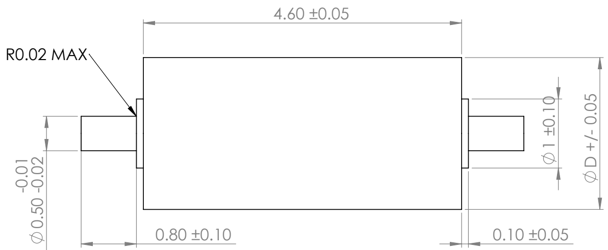
Figure B.2. Technical drawing of 3-DOF PRD's rollers. D is 2.20 mm and 1.40 mm for outer and inner rollers respectively. All dimensions are in mm.
