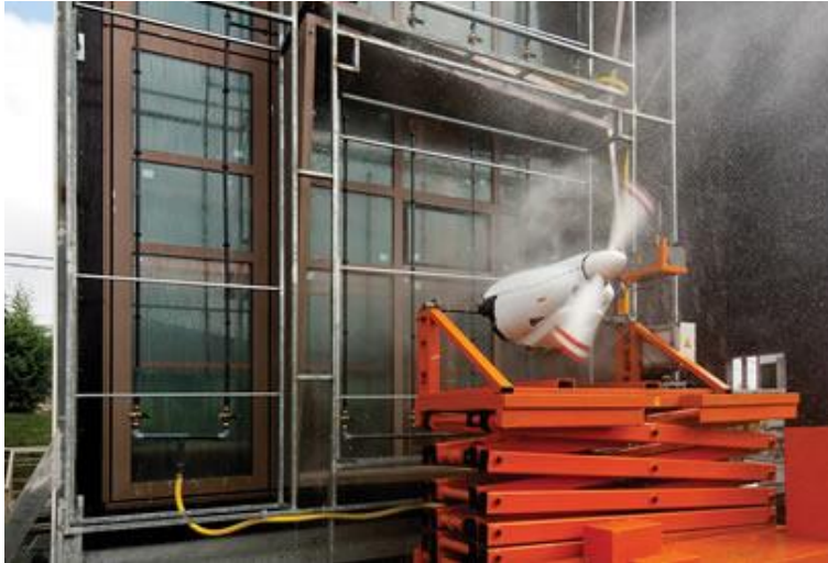
Figure 3.11 : Test setup for facade performance evaluation (Url-30).
