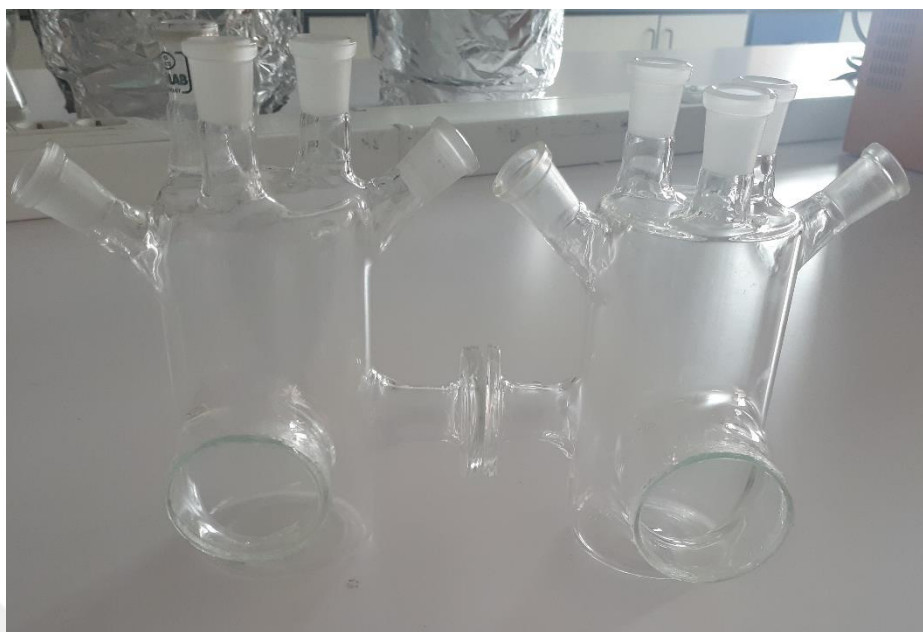
Figure 3.3. The designed photo reactor.
