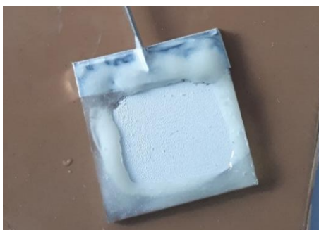
Figure 3.1. Un-doped \text{SrTiO}_3 prepared by SSR, coated by doctor blade.
