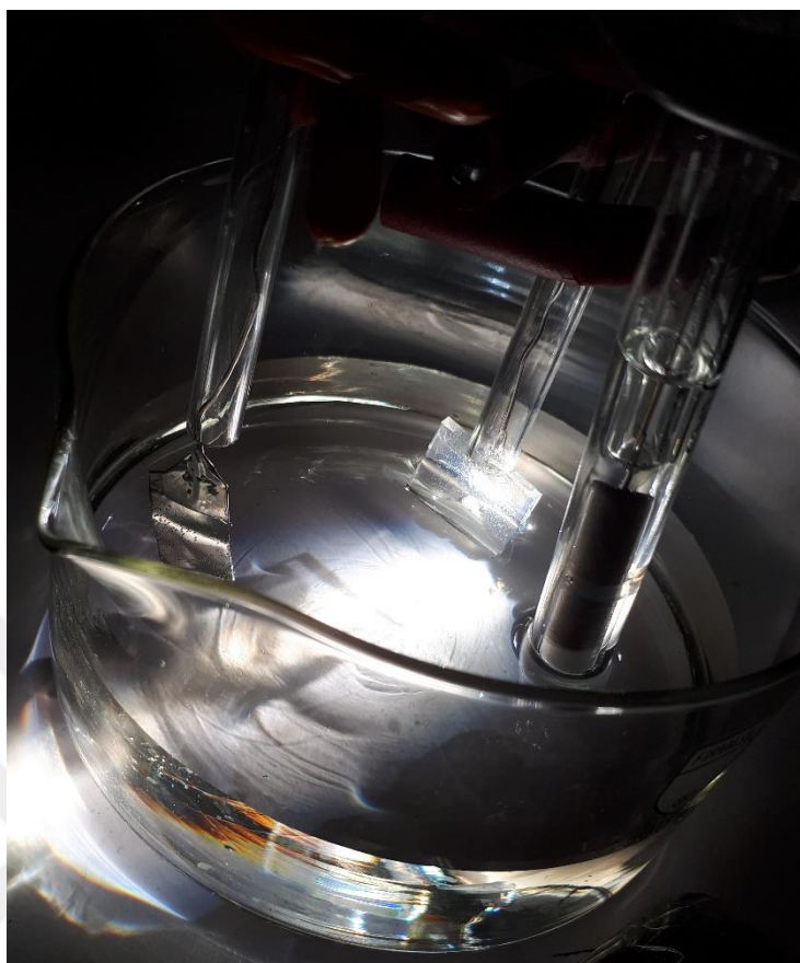
Figure 3.4. The open beaker photoelectrochemical setup for three electrode configuration.
