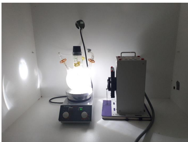
Figure 3.5. The setup of photocatalytic water splitting.
