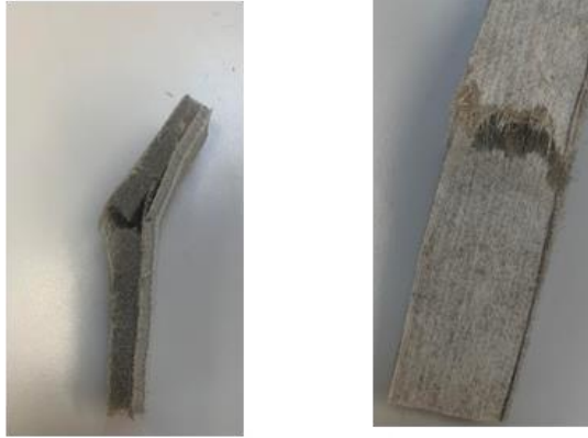
Figure 4.3: A permanent deformation on FL1 & FL3 samples after a tensile test.
