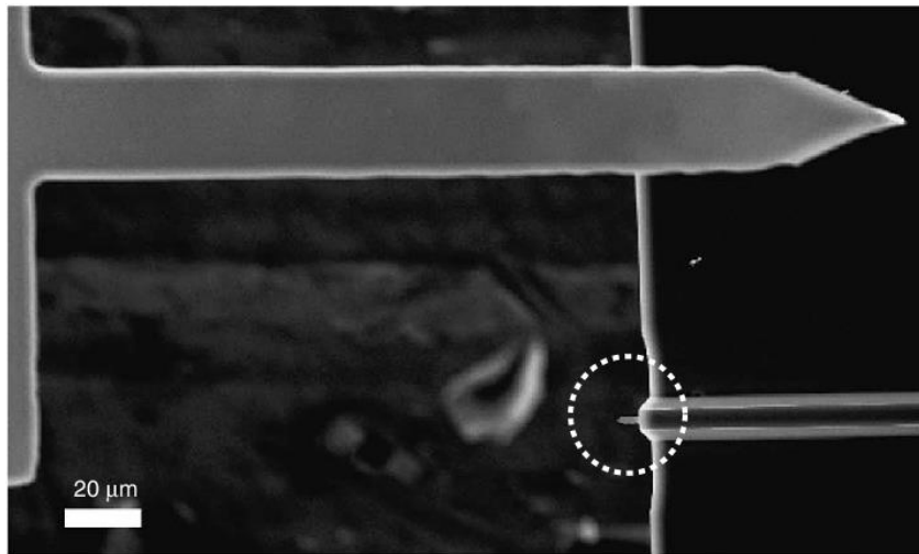
Figure 2.3. “SEM micrograph of a conventional AFM cantilever (Olympus OMCL-AC240TS) and a small cantilever (Olympus BL-AC10DS; encircled)” [41]
