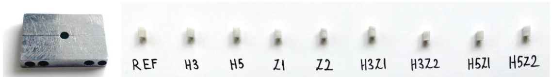
Figure 3.7 Two-piece stainless steel mold and prepared compression test specimens
