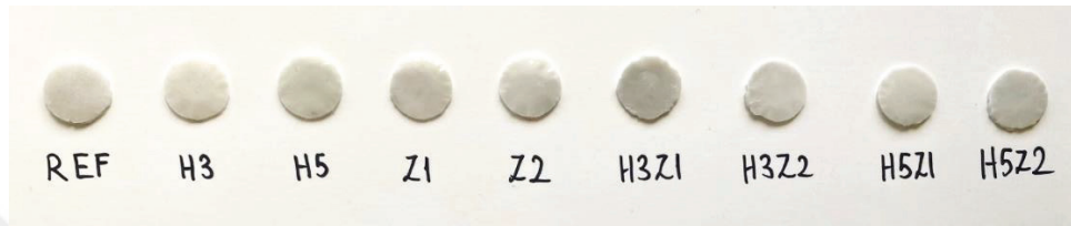
Figure 3.9 Water sorption and solubility test specimens
