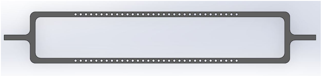
Figure 4.2: Schematic of an MZI with Photonic Crystal Waveguides.
