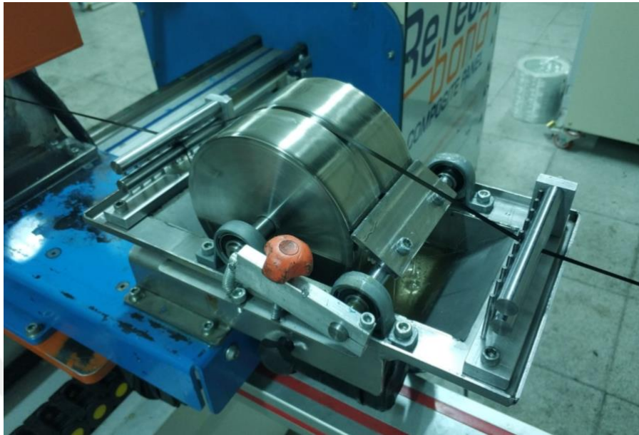
Figure 3.5. Impregnation of carbon fibers within resin bath
