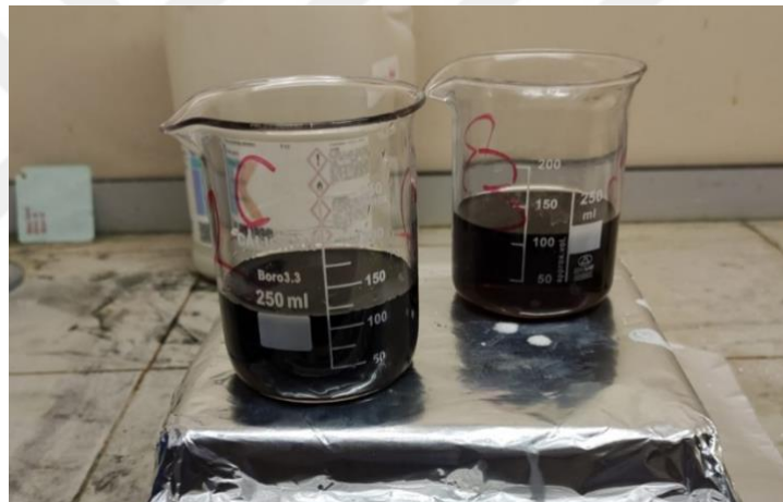
Figure 3.21. Acid digestion process of two samples before hydrogen peroxide addition
