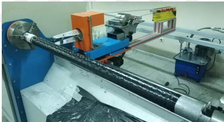
Figure 3.6. The completed filament-wound carbon fiber tube
