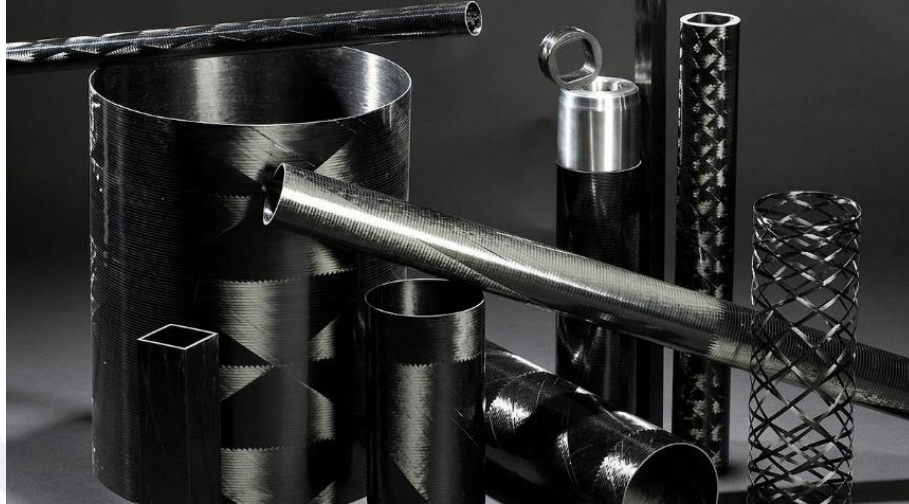
Figure 1.4. Filament winding axisymmetric examples (Source: Mateduc Composites)
