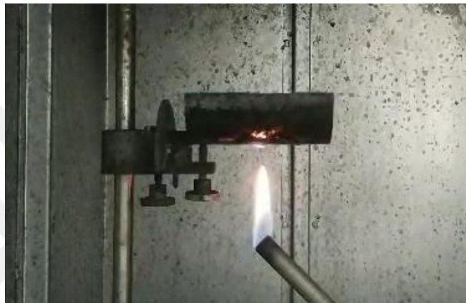
Figure 4.19. Half tube sample during flammability test
