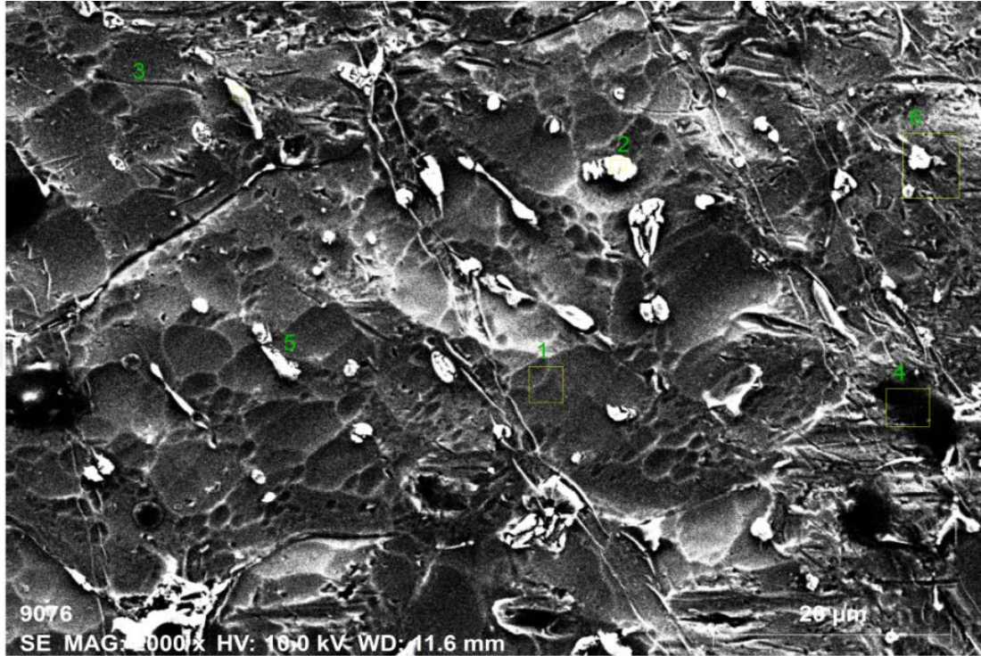
Figure 4. 8. SEM image of 2024 Al alloy/3 wt. % Micro and Nano Y_2O_3
