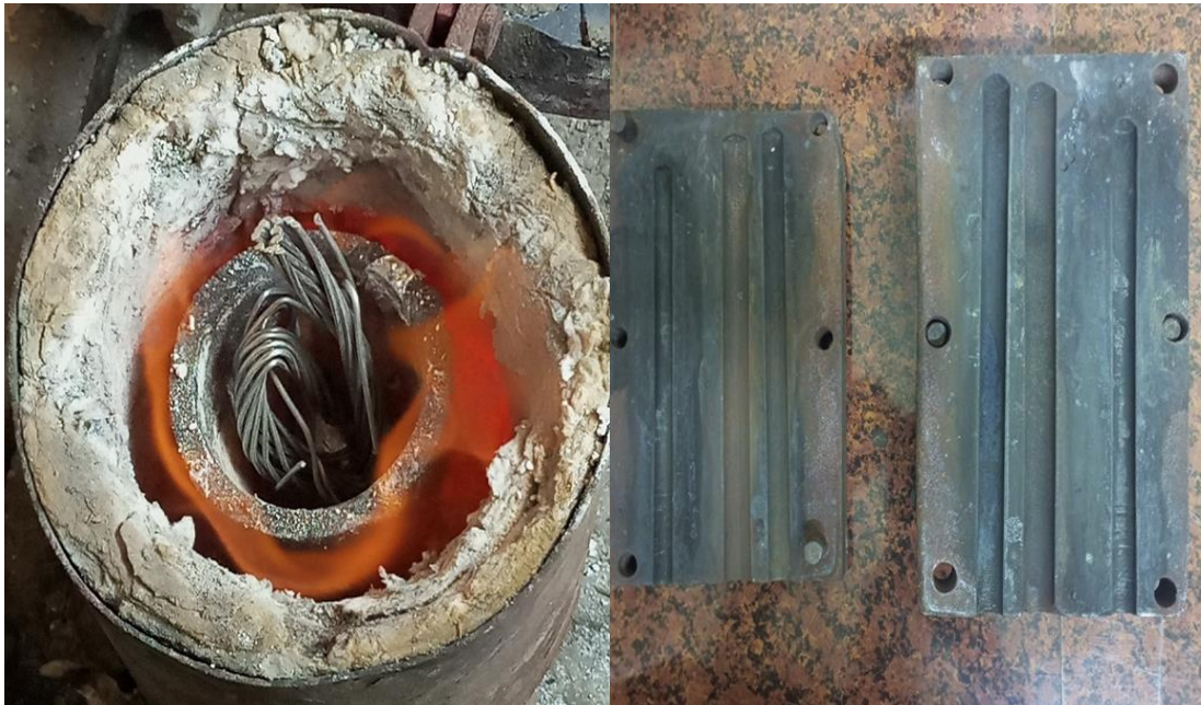
Figure 3.5. Casting mould, melting crucible and gas furnace.
