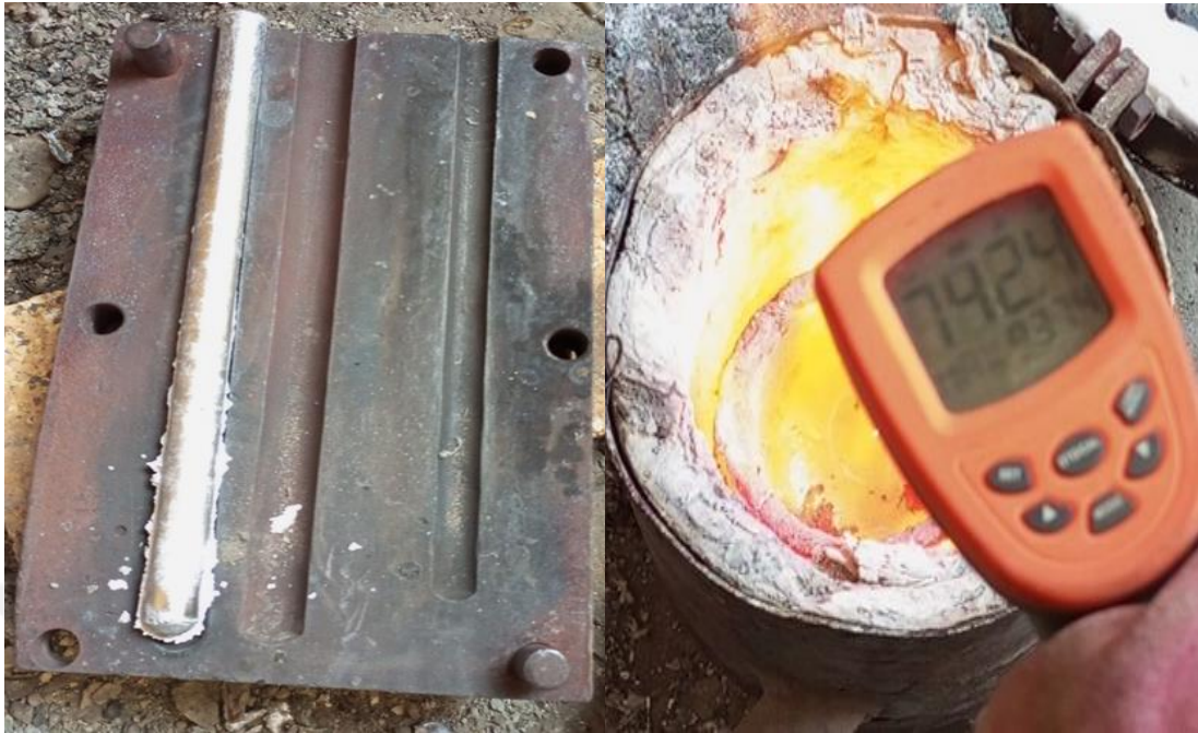
Figure 3.6. Casting temperature scale and the special model for making test samples
