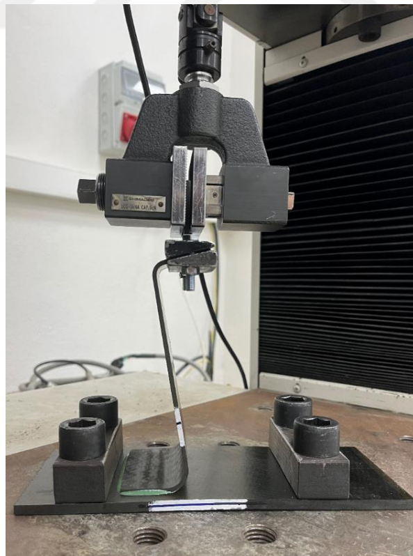
Figure 33. Image from SSJ joint specimen test moment.
