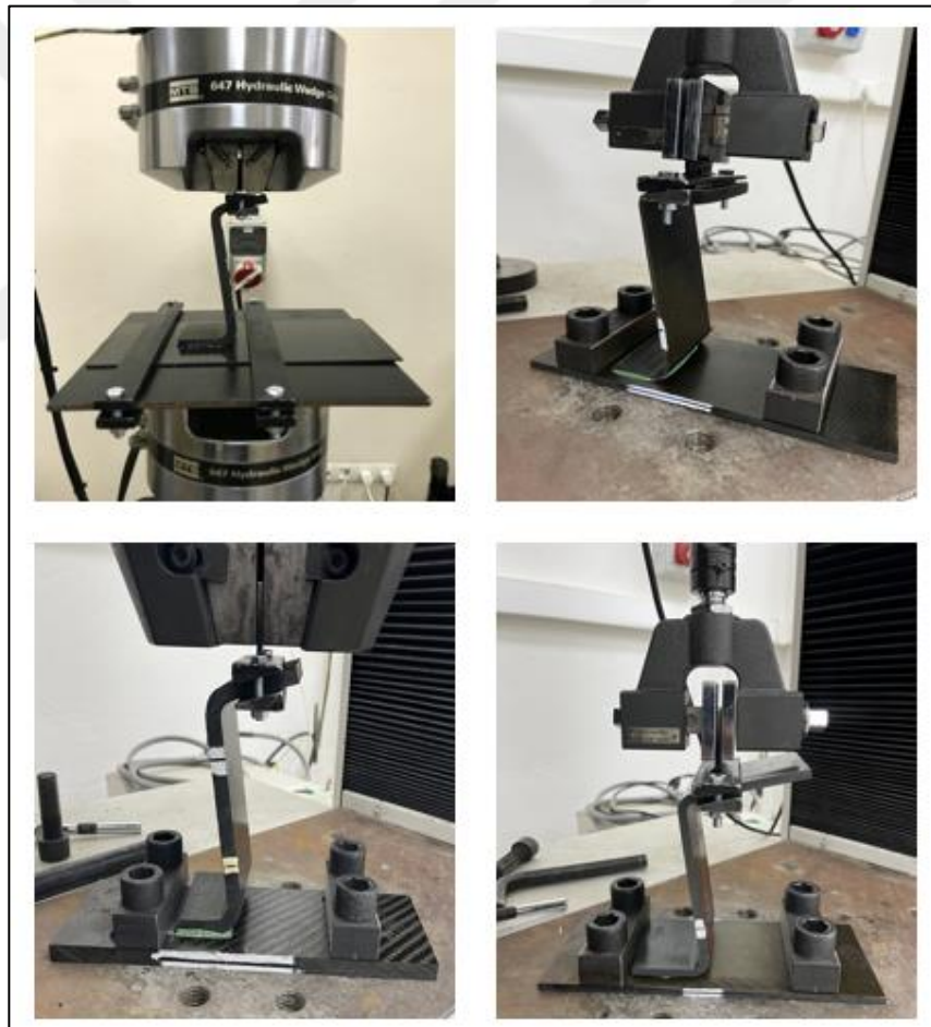
Figure 30. Various SSJ test setups, specimens and configurations have been tried.
