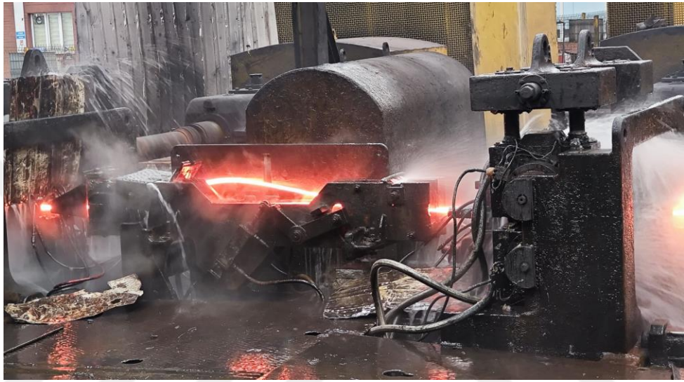
Figure 3.8. Loop formation in hot rolling mill.
