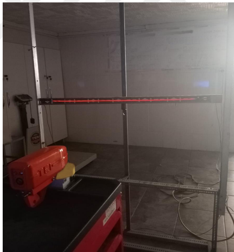
Figure 5.15. Loop scanner detecting resistance wire.
