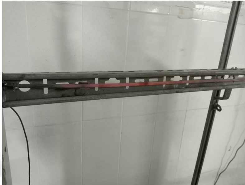
Figure 5.14. Resistance wire used in mechanical setup.
