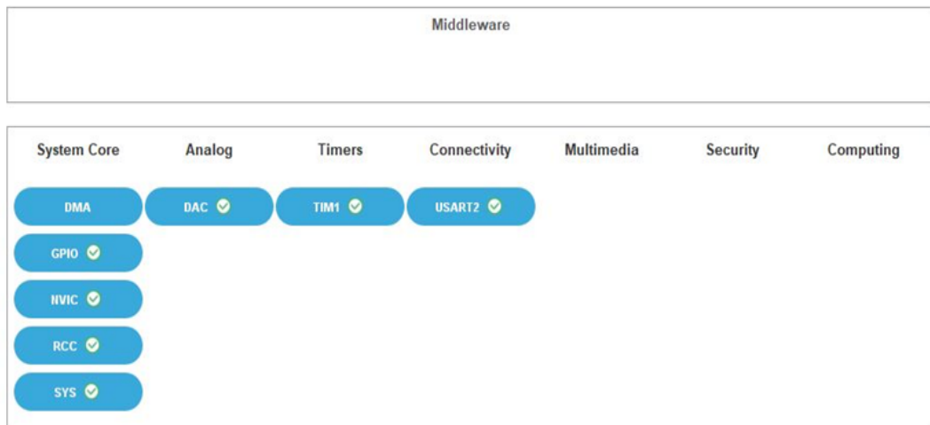
Figure 5.9. STM32 CubeMX middleware config.
