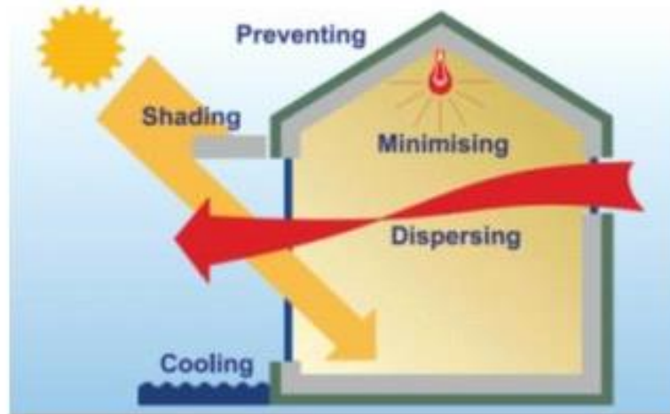
Figure 12: An illustration of Bioclimatic strategies for cooling in buildings (Liebard et al, 2005.)
