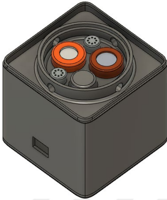
Figure 3.7. The sensor chamber and body of the test device with added 5 sensors.
