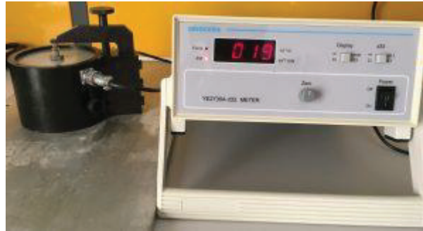
Figure 1.27. Room temperature piezoelectric d_{33} coefficient measurement tool; d_{33} Meter (SINOCERA YE2730A).
