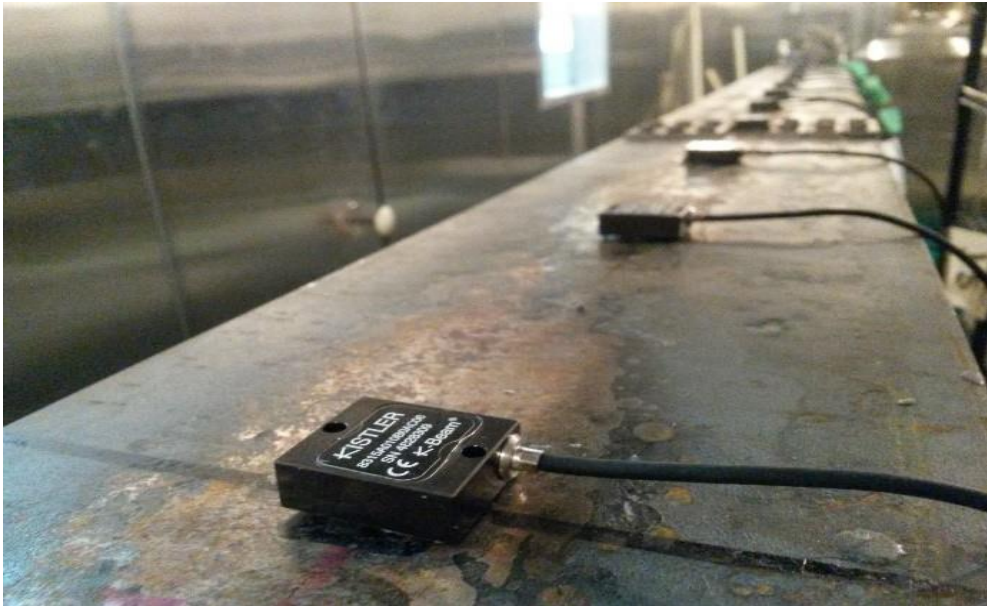
Figure 2.1: Accelerometers of Structure Health Monitoring (Roberts et al, 2004).
