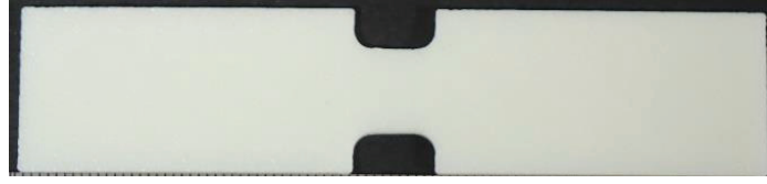
Figure 21 Custom ABS specimen that is printed using FDM method for dynamic tensile testing.
