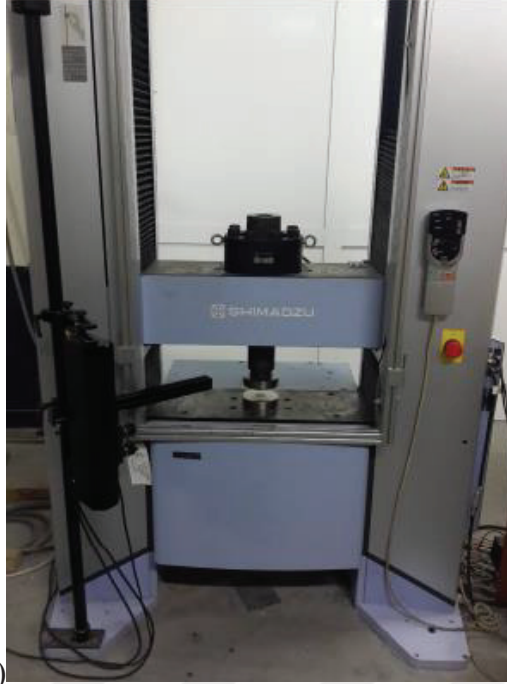
Figure 24 Quasi-static a) tension b) compression test set-up
