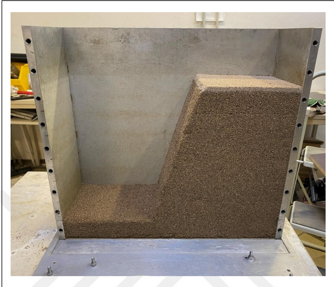
Figure 4.8 : Slope model in the box.
