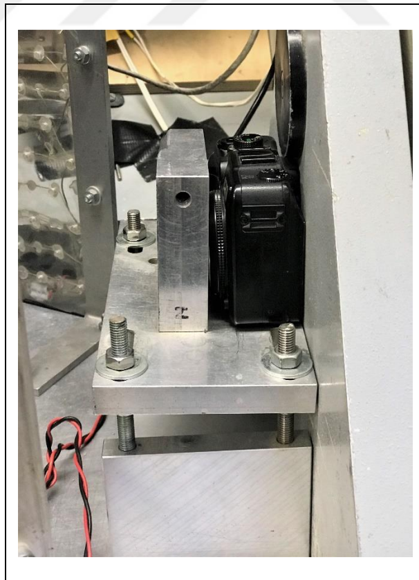
Figure 4.11 : Assembling the digital camera in front of the model box.
