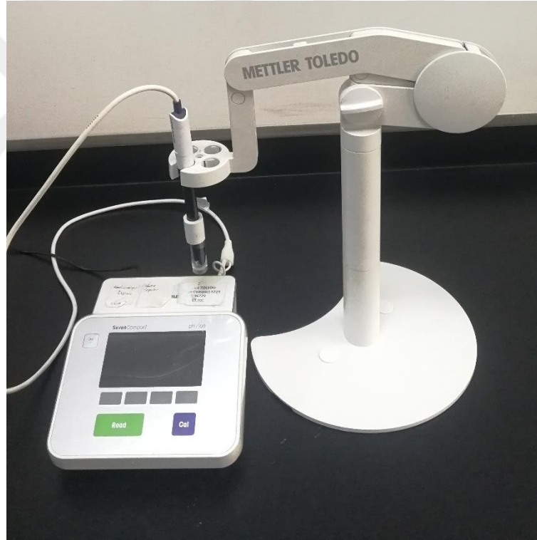
Şekil 3.1 : Dijital pH metre (Mettler Toledo Orion Seven Compact S220).
