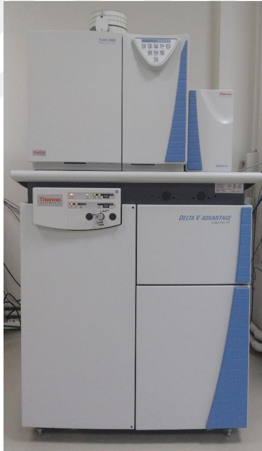
Şekil 3.14 : İzotop Oranı Kütle Spektrometre Sistemi (IR-MS) (Thermo Scientific Flash 2000 Organic Elemental Analyzer & Delta V Advantage Isotope Ratio MS).
