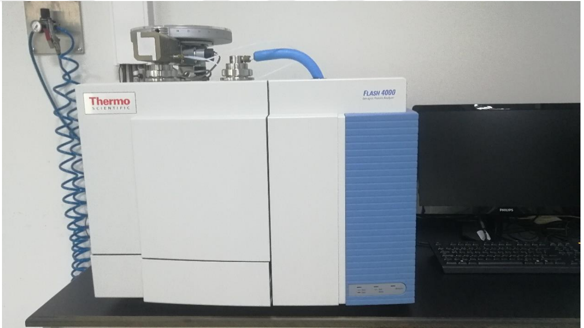
Şekil 3.4 : Azot/protein tayin cihazı (Thermo Scientific Flash 4000).
