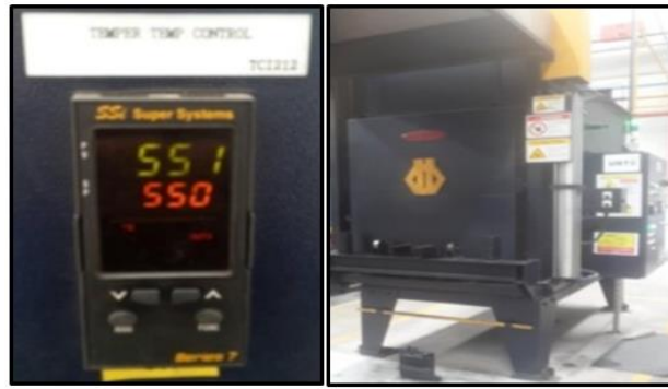
Figure 23. Used AFC Holcroft CQI9 brand heat treatment furnace
