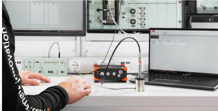
Figure 2.27 : A comparison method setup for microphone calibration [66].
