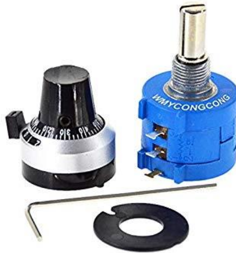
Figure 2.28 : Adjustable multi turn potentiometer [67].
