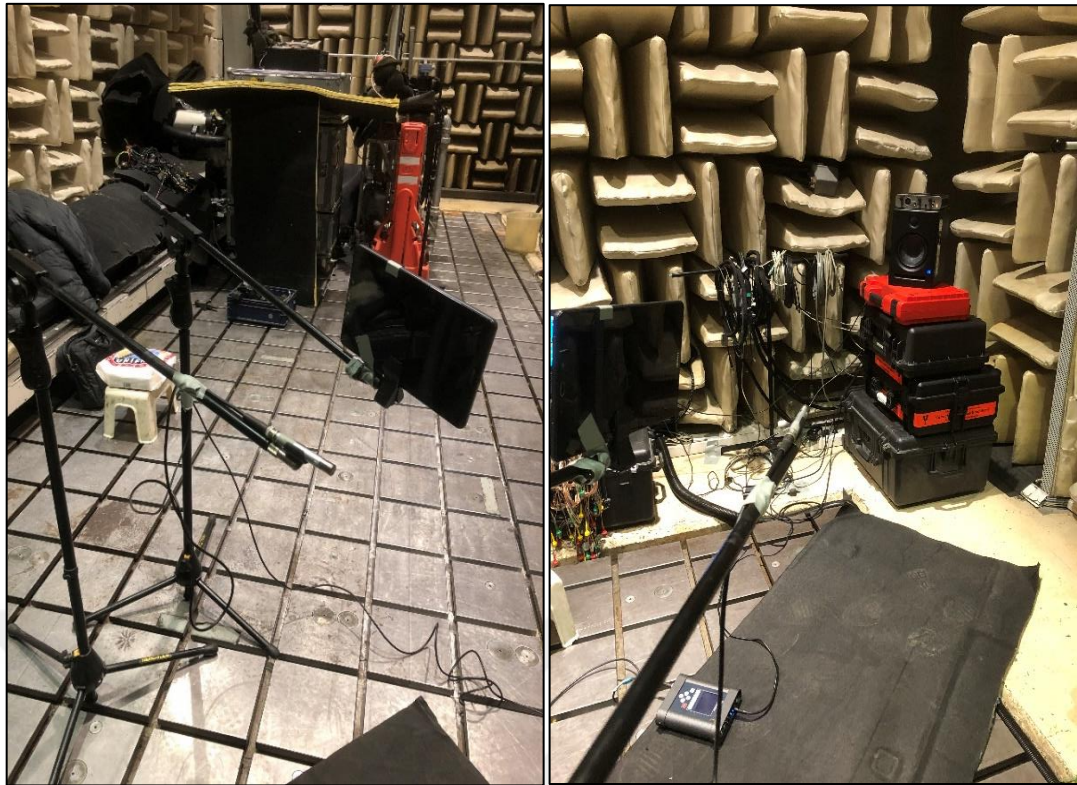
Figure 3.5 : The initial test setup for hemi anechoic room measurements.
