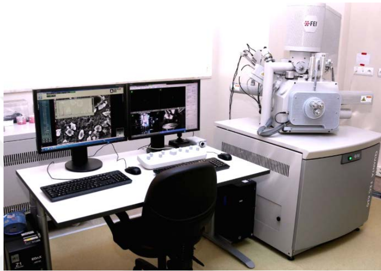
Figure 3.5. EDS integrated FEI Quanta FEG-650 model scanning electron microscope.
