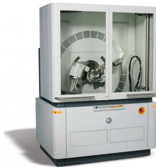
Figure 3.3. PANalytical EMPYREAN X-ray diffraction (XRD) system.
