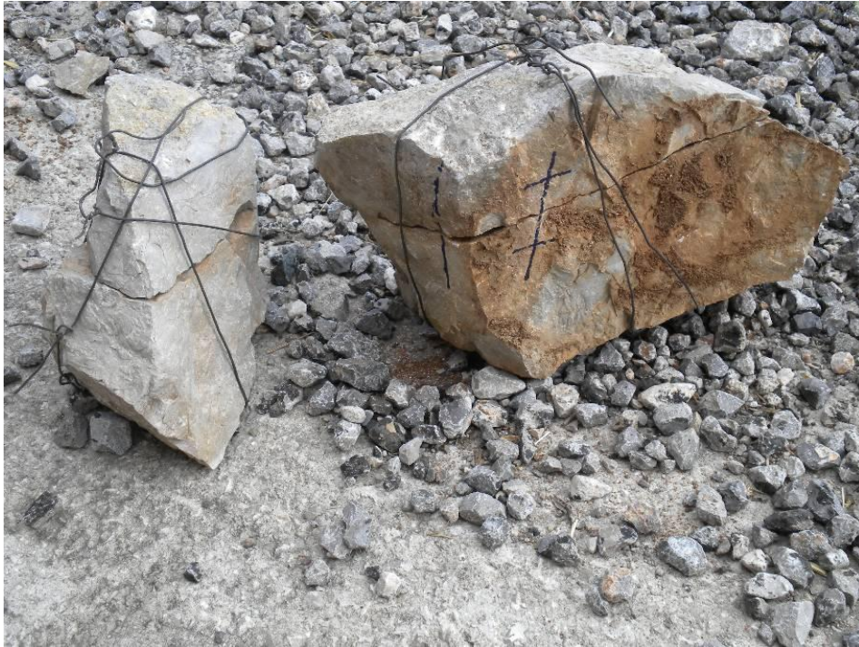
Figure 3.4. Photograph of the oriented samples taken from the field.
