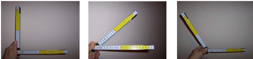
Figure 3.8 Constructing Different Angles with Mason Ruler
