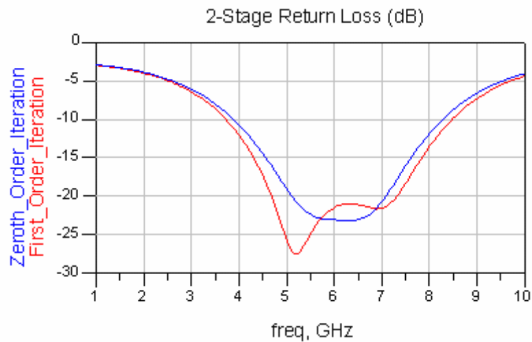
Figure 3-60: EM Simulation Result of 2-stage Matching Section Design
