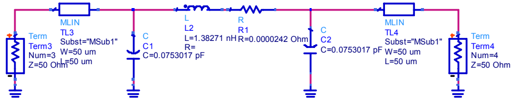
Figure 4-24: Circuit Model Schematic of Spiral Inductor with Dimensions 510x510 \mu\text{m} and 1 \frac{3}{4} Turn
