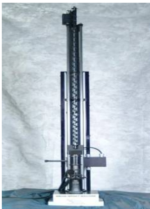
Figure 2.1. The impact sensitivity test apparatus.
