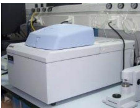
Figure 2.4. Differential Scanning Calorimetry (DSC).
