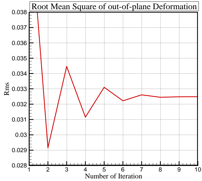
Figure 3.26 The Root Mean Square of out-of- plane Deformation at Each Aeroelastic Time-step
