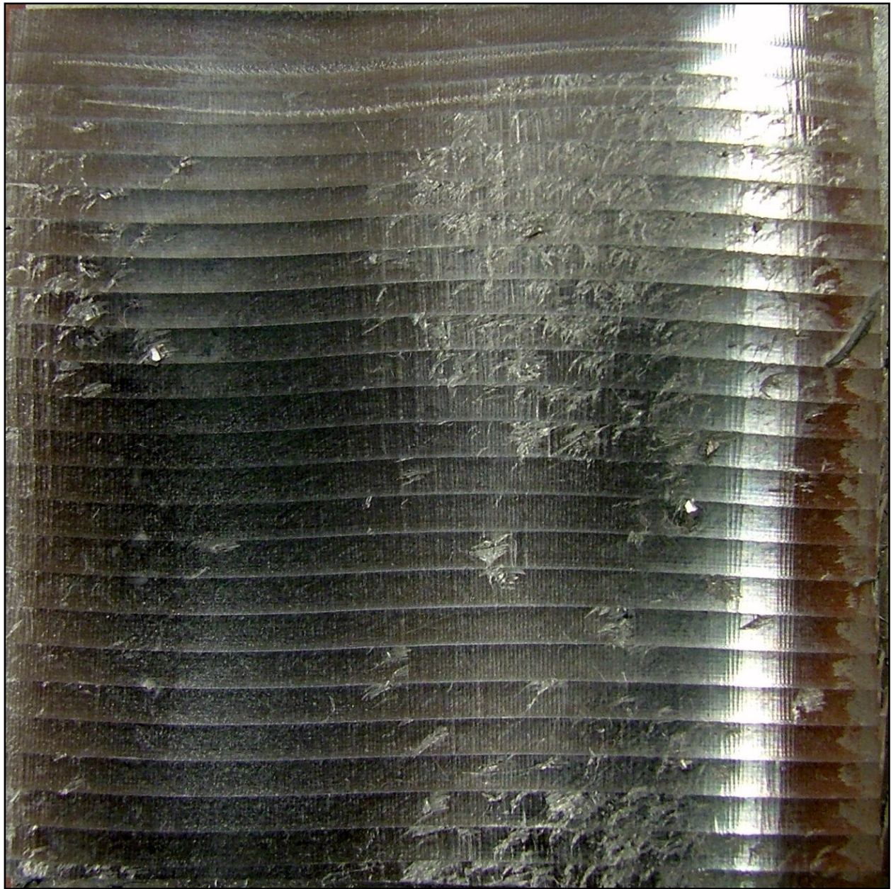
Figure 8.17: Surface quality of -30^\circ tilt angle sine – cosine surface.
