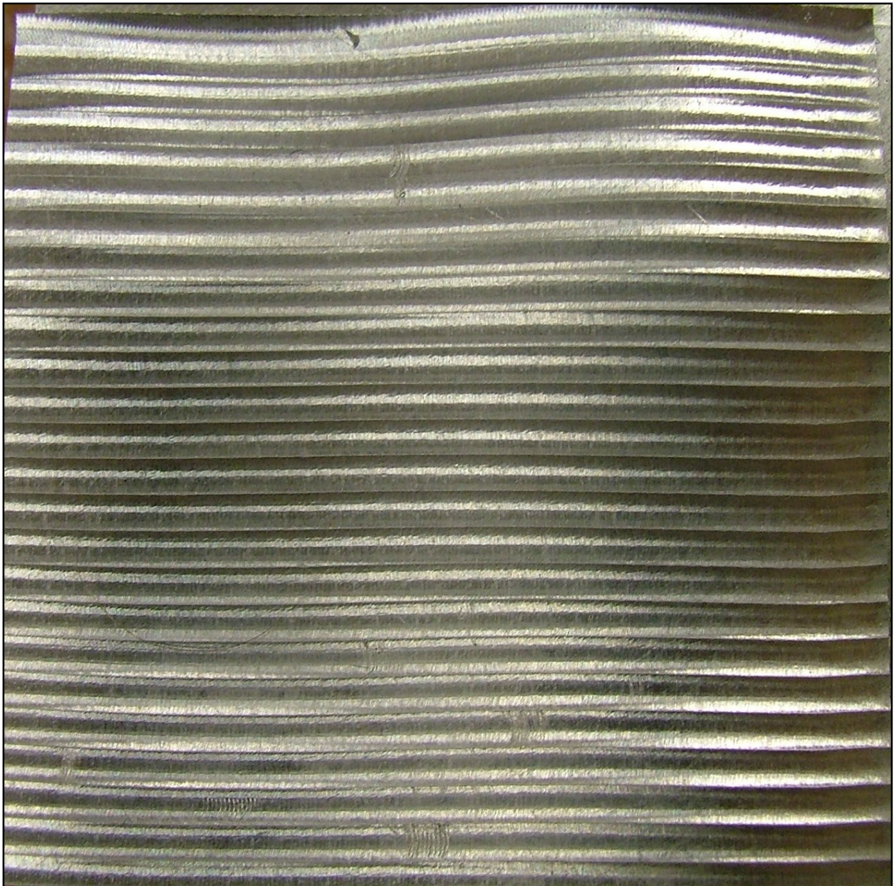
Figure 8.14: Surface quality of 30° lead angle sine – cosine surface.
