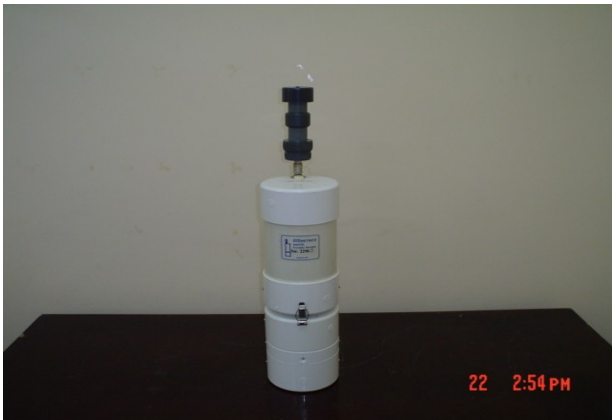
Figure A.2: Airmetrics Minivol Portable Air sampler. The parts are joined to form the block.
