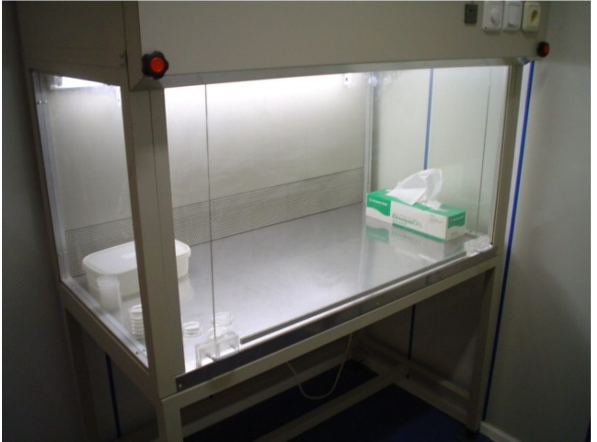
Figure A.10: The clean hood.
