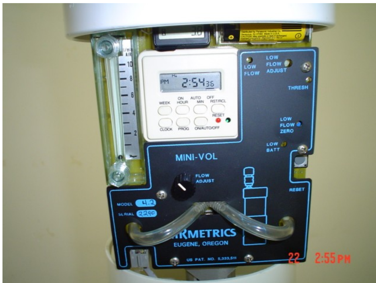
Figure A.3: The Program Control Unit of the Airmetrics Minivol Portable Air sampler. (The flow meter, programmable timer and the flow adjustment units)
