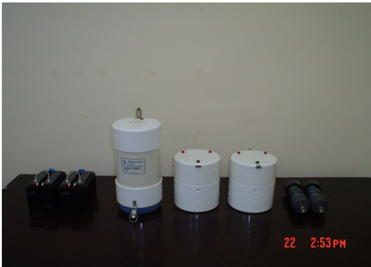
Figure A.1: Airmetrics Minivol Portable Air sampler. Each part separately shown: Two batteries, the main block, two battery cases and two filter heads.
