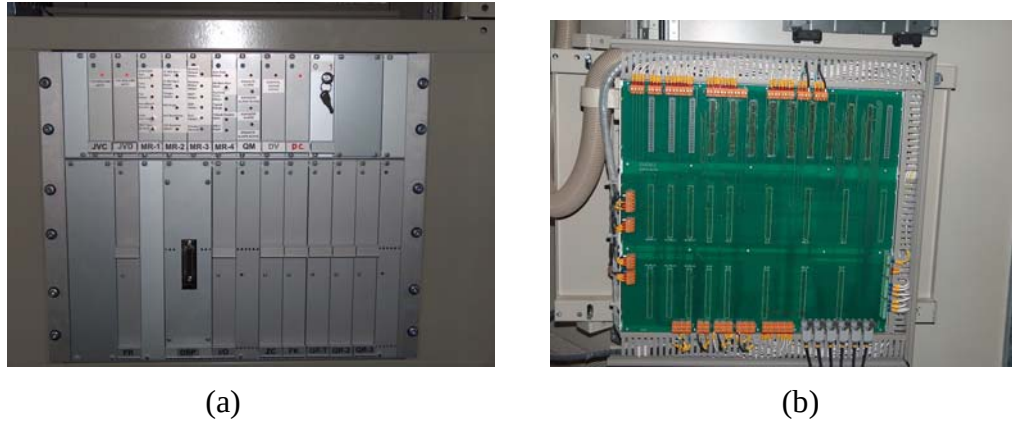
Figure 3.53 Picture of electronic system for CSC based STATCOM (a) front view (b) view of motherboard
