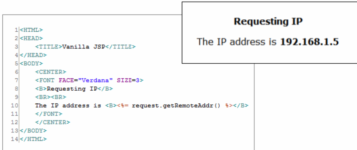
Figure II.3. A JSP page with HTML layout tags embedded in it
