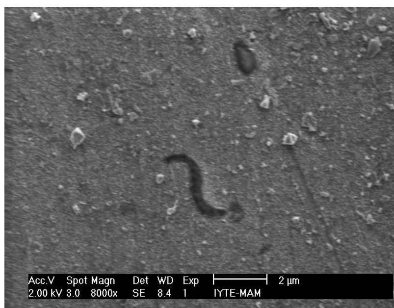
Figure 4.35. SEM image of a sulphate reducing bacterium.
