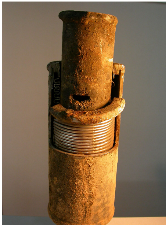
Figure 2.15. Corrosion caused by the galvanic effect on a compensators taken from Balçova-Izmir geothermal system.
