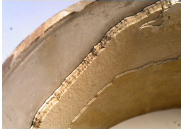
Figure 1.8. Stainless steel pipe scaling layer section
