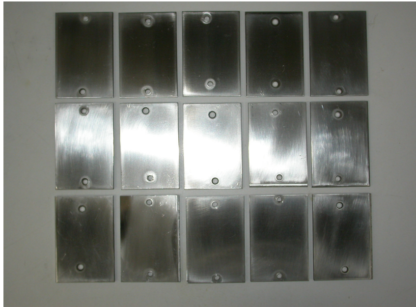
Figure 3.6. Austenitic stainless steel corrosion test coupons.
