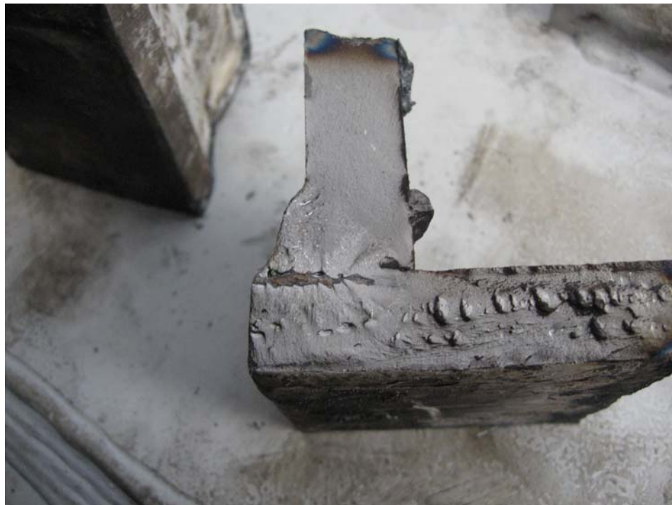
Figure 3.9 Failed parts of an excavator boom
