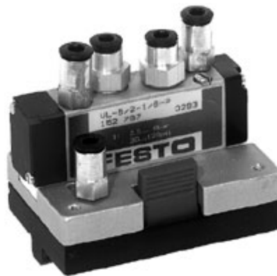
Figure 2.4 5/2-way double control valve, pneumatically actuated, by boost chambers on each side of the spool. ( Festo, J type valves)
