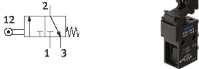
Figure 2.7 3/2 valve with roller lever control. (Festo AR type valves, R standing for “Roller” )
