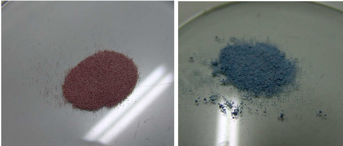
Figure 4.5. m-PHEMA/PEI beads before and after incubation with \text{Cu}^{2+} solution.
