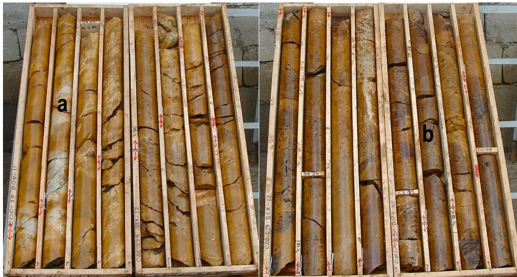
Figure 2.14 Core photo from the Marble Contact Zone, CDD-039,45.9-60.6 m. Oxidized intrusive (a) and gossan (b).
