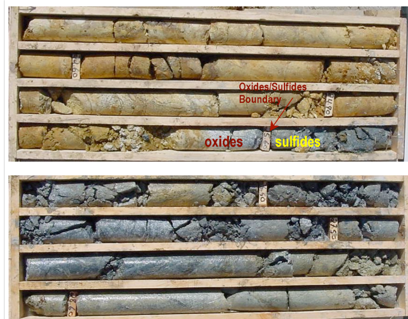
Figure 2.12 Photography of the core sample from Main zone sample no: CDD-002; between 21.5 to 29.4 m. Oxide / Sulphide boundary shown at 25.45 m (Poyraz, 2005)
