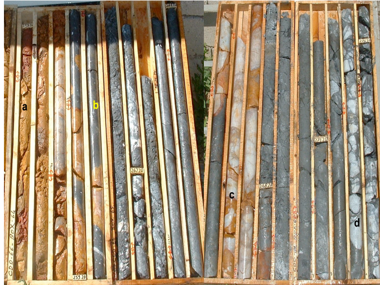
Figure 2.13 Photography of the core sample from Mn Mine Zone – Oxide (a) and Sulphide (b) Mineralization. Core samples: CDD-066, CDD 256-5-274.35 m. Marble breccia (c) and argillized brecciated intrusives (d).
