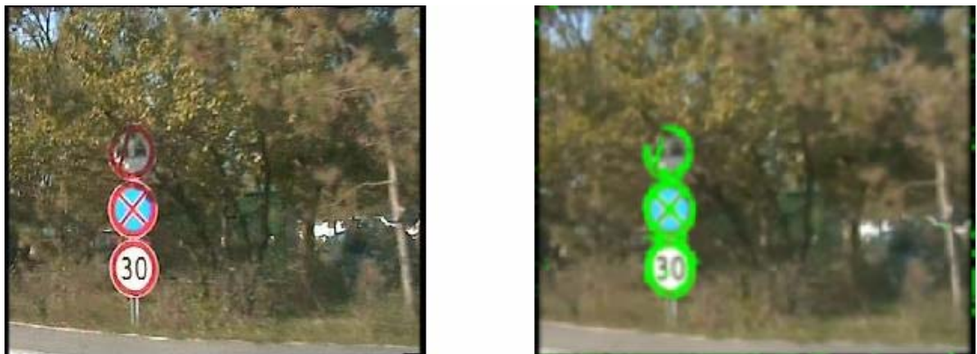
Figure 3.18: A traffic scene on left and red-color emphasized image on right
