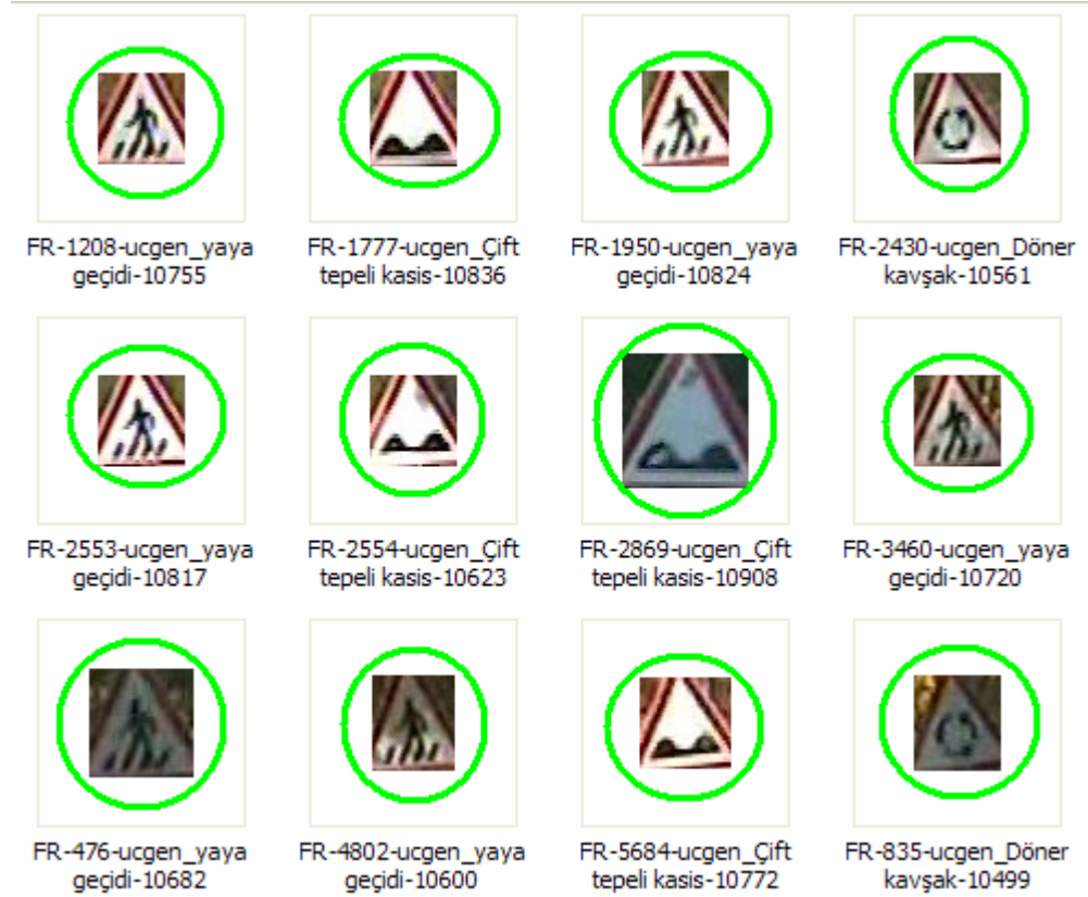
Figure 5.4: Detected and recognized triangular signs for Parameter Set-1 and Threshold Set-2 (5 levels) for Table 5.8
