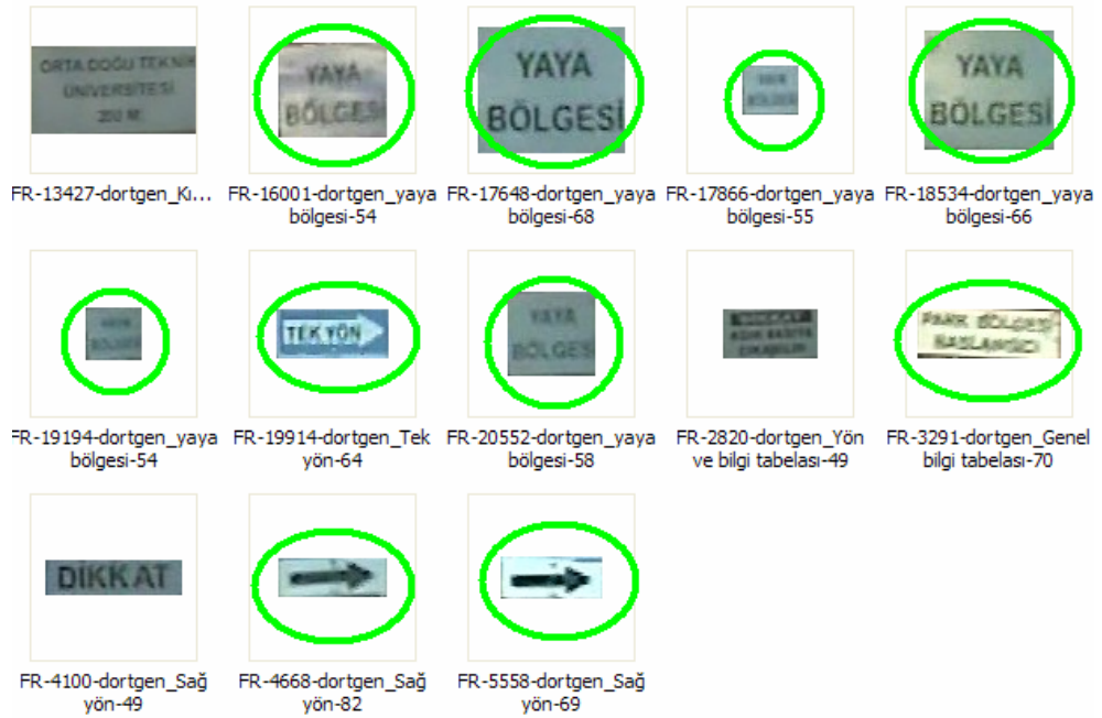
Figure 5.70: Detected and recognized rectangular signs for parameter Set-1 and Threshold Set-3 (3 levels) for Table 5.42.
