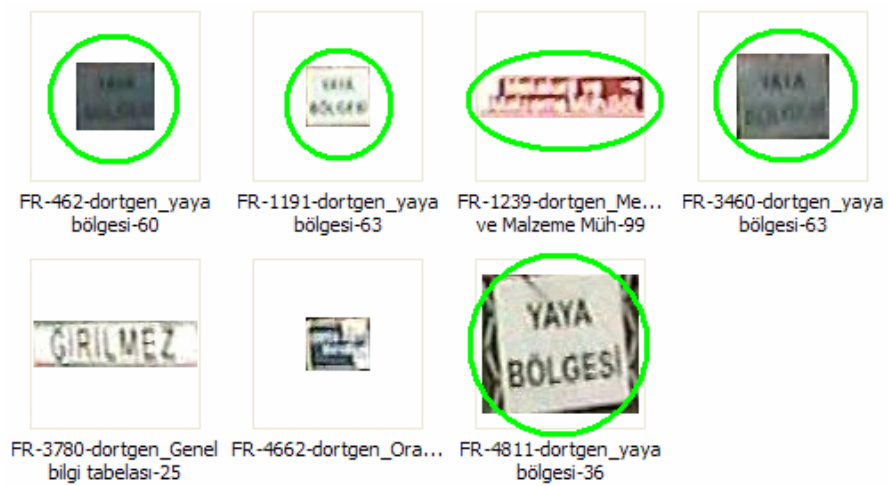
Figure 5.9: Detected and recognized rectangular signs for Parameter Set-1 and Threshold Set-3 (3 levels) for Table 5.9
