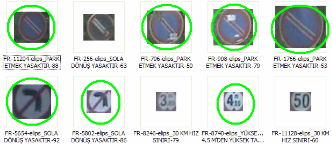
Figure 5.52: Detected and recognized circular signs for parameter Set-1 and Threshold Set-2 (5 levels) for Table 5.35.
