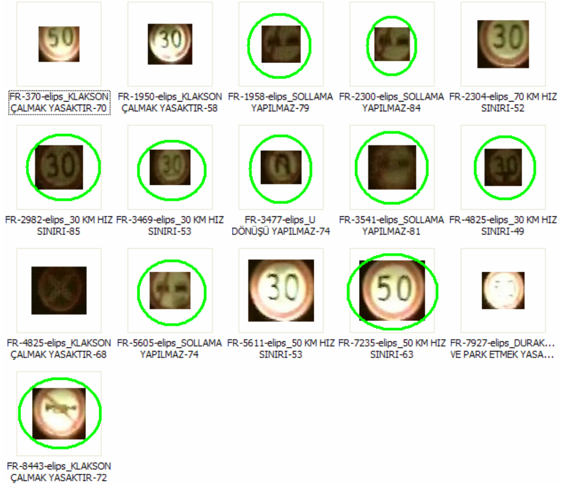
Figure 5.45: Detected and recognized circular signs for parameter Set-4 and Threshold Set-2 (5 levels) for Table 5.29
