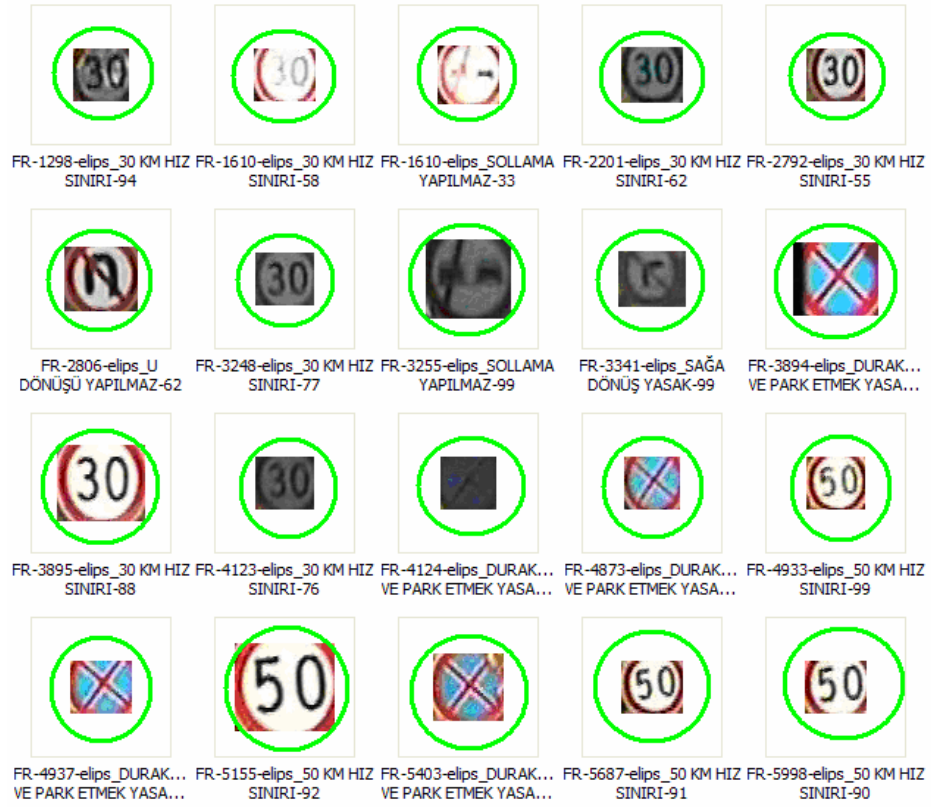
Figure 5.17: Detected and recognized circular signs for Parameter Set-4 and Threshold Set-3 (3 levels) for Table 5.12
