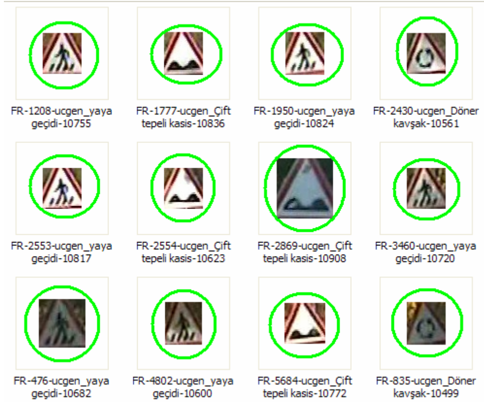
Figure 5.1: Detected and recognized triangular signs for Parameter Set-1 and Threshold Set-1 (10 levels) for Table 5.7
