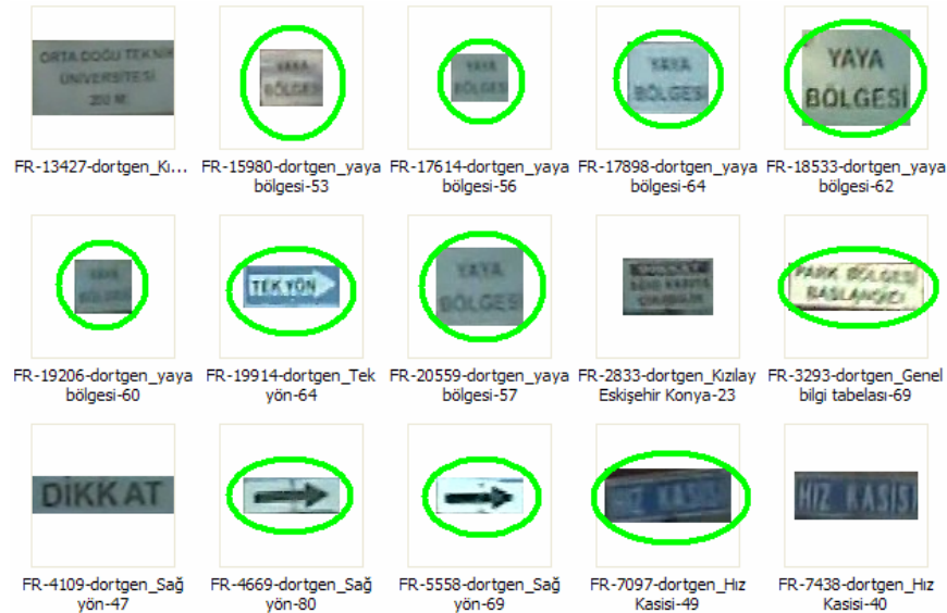
Figure 5.66: Detected and recognized rectangular signs for parameter Set-1 and Threshold Set-2 (5 levels) for Table 5.41.
