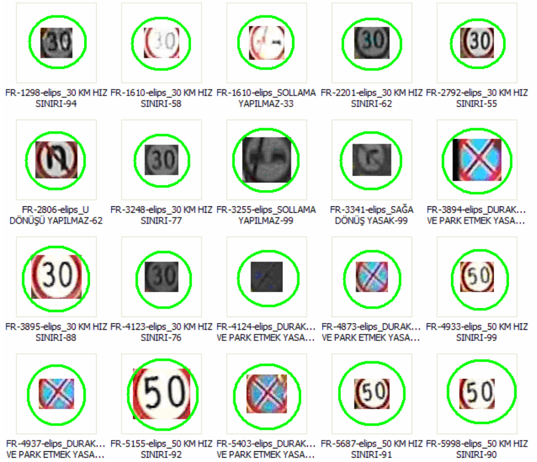
Figure 5.11: Detected and recognized circular signs for Parameter Set-4 and Threshold Set-1 (10 levels) for Table 5.10
