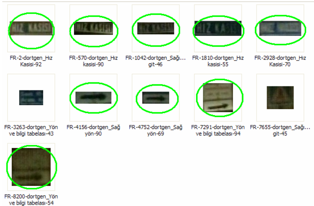
Figure 5.33: Detected and recognized rectangular signs for Parameter Set-2 and Threshold Set-1 (10 levels) for Table 5.22
