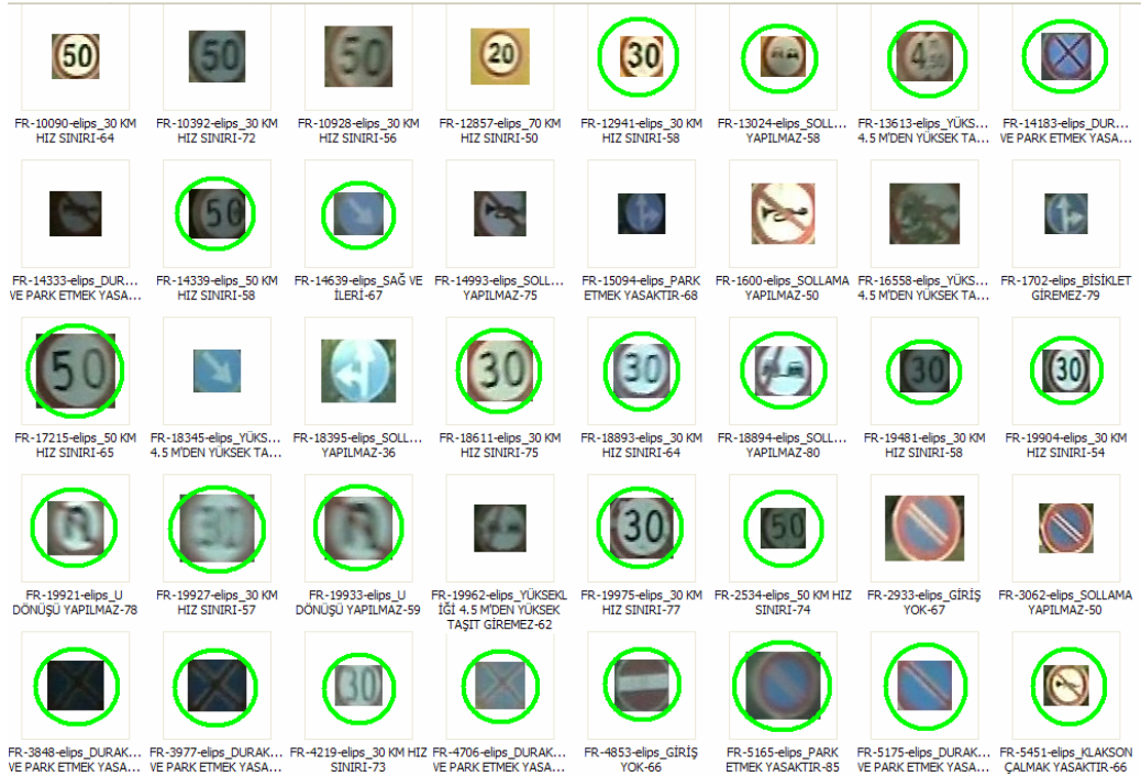
Figure 5.60: Detected and recognized circular signs for parameter Set-1 and Threshold Set-1 (10 levels) for Table 5.40.
