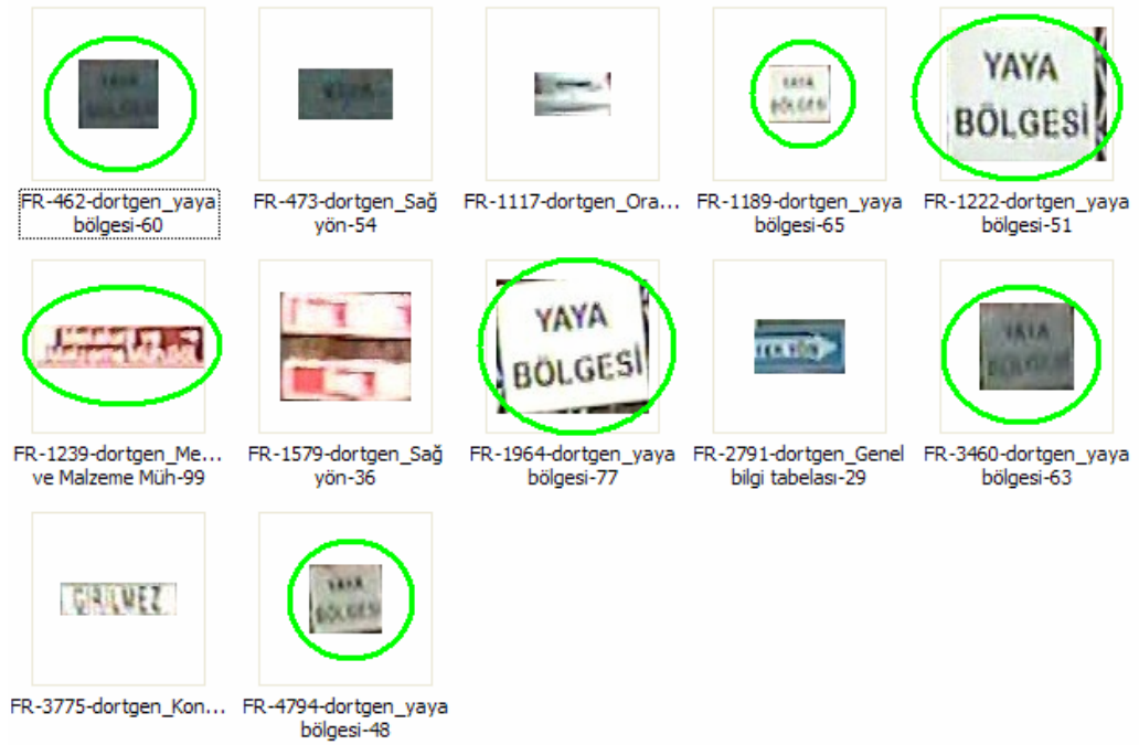
Figure 5.12: Detected and recognized rectangular signs for Parameter Set-4 and Threshold Set-1 (10 levels) for Table 5.10
