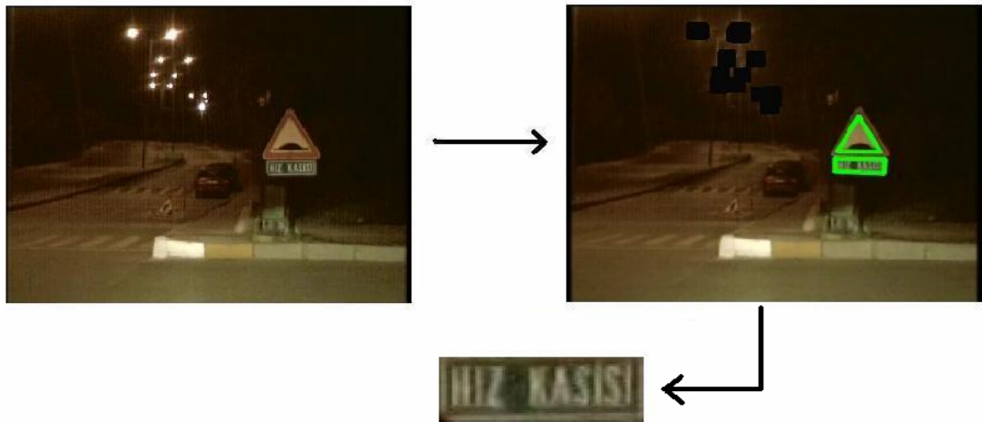
Figure 3.10: Detected rectangular and triangular signs taken at night with cropped rectangular sign
