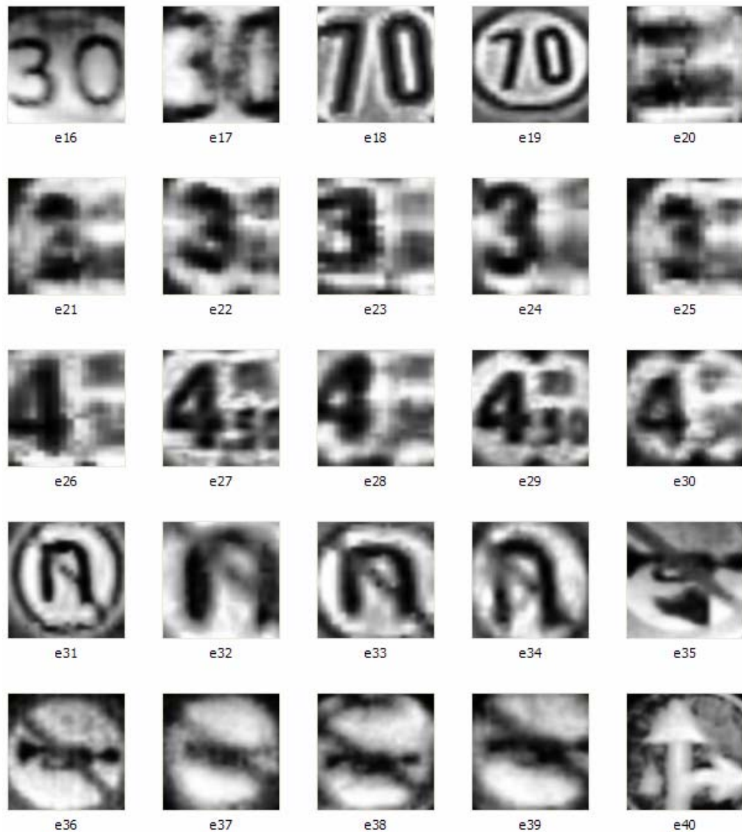
Figure 4.17: Examples of circular sign template database
