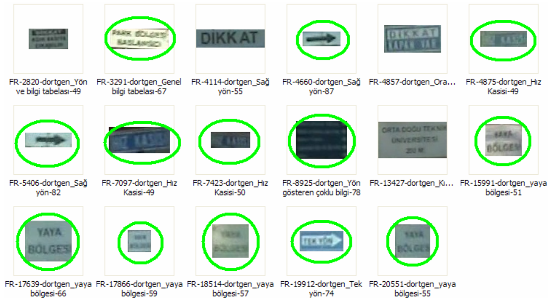
Figure 5.62: Detected and recognized rectangular signs for parameter Set-1 and Threshold Set-1 (10 levels) for Table 5.40.
