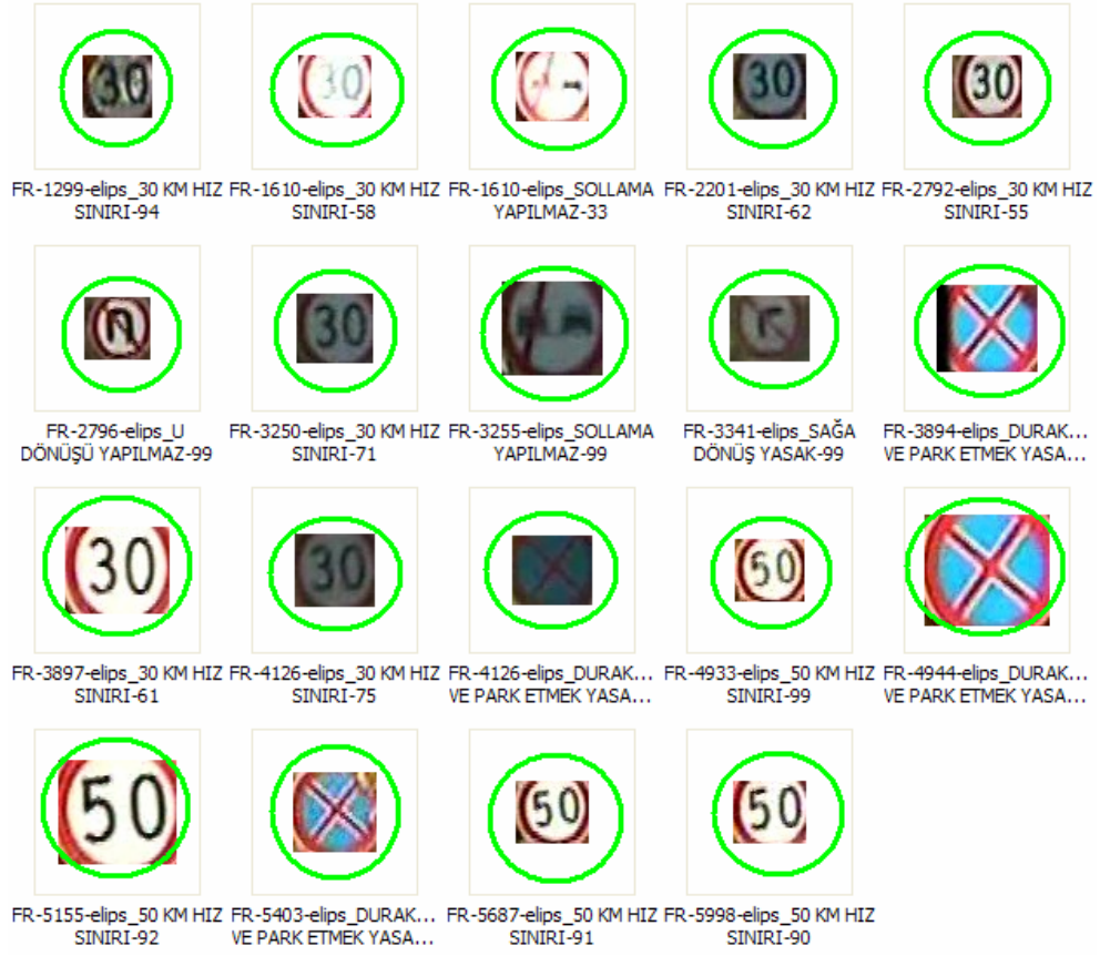
Figure 5.5: Detected and recognized circular signs for Parameter Set-1 and Threshold Set-2 (5 levels) for Table 5.8
