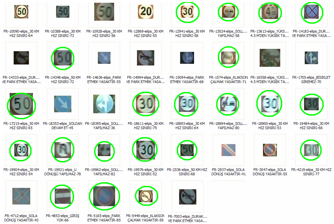
Figure 5.64: Detected and recognized circular signs for parameter Set-1 and Threshold Set-2 (5 levels) for Table 5.41.
