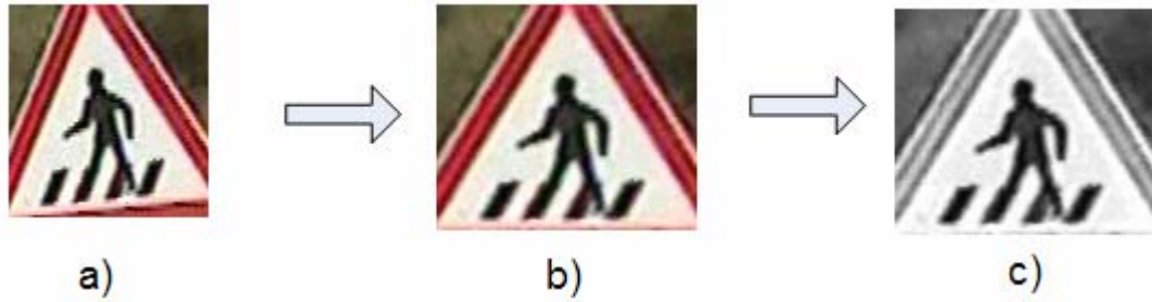
Figure 4.6: (a) Detected and cropped traffic sign candidate, (b) transformed, RGB color image, (c) V channel of HSV equivalent transformed image
