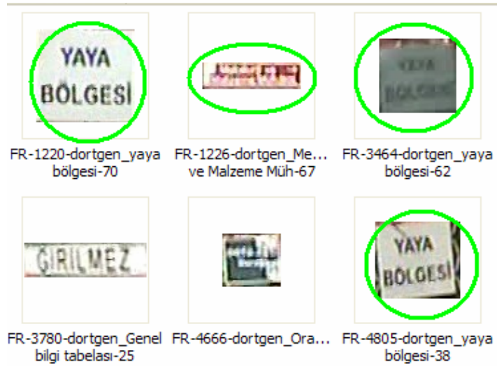
Figure 5.18: Detected and recognized rectangular signs for Parameter Set-4 and Threshold Set-3 (3 levels) for Table 5.12
