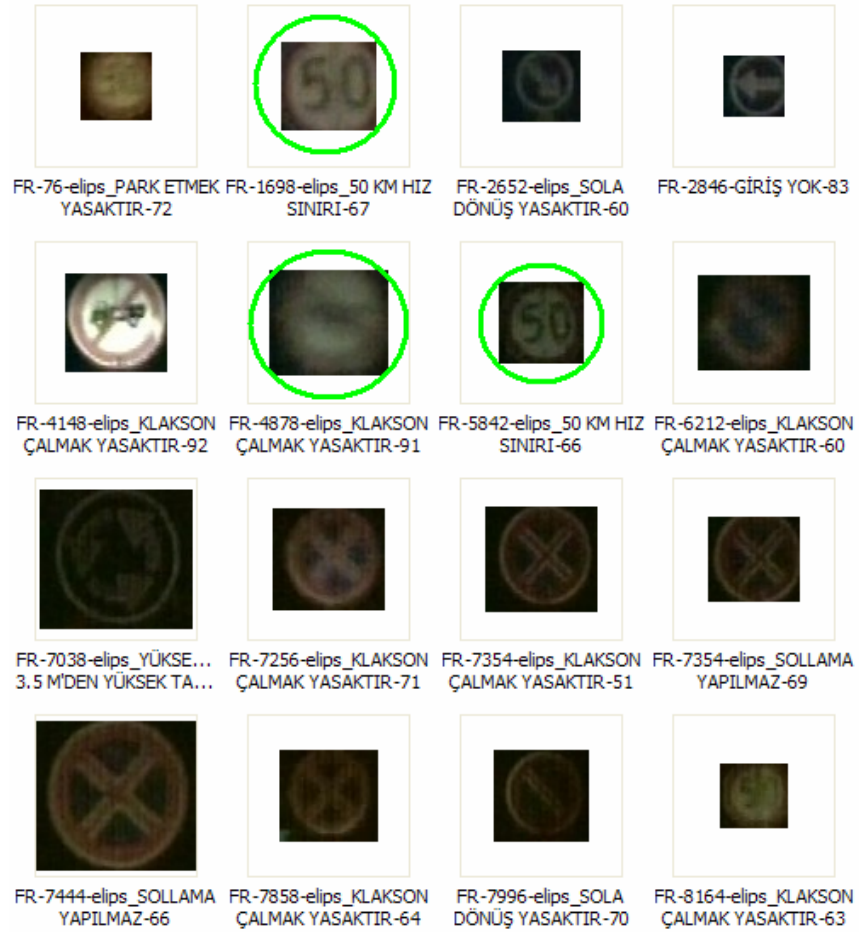
Figure 5.24: Detected and recognized circular signs for Parameter Set-3 and Threshold Set-2 (5 levels) for Table 5.20
