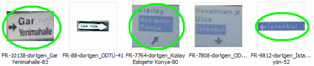
Figure 5.54: Detected and recognized rectangular signs for parameter Set-1 and Threshold Set-2 (5 levels) for Table 5.35.
