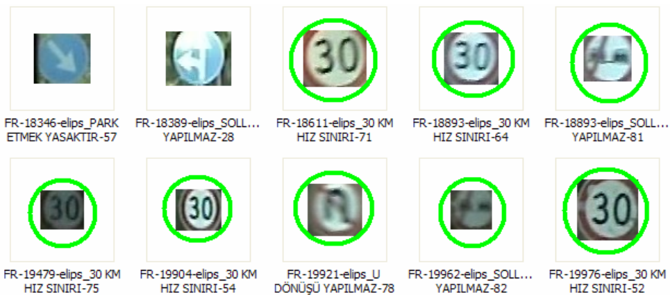
Figure 5.68: Detected and recognized circular signs for parameter Set-1 and Threshold Set-3 (3 levels) for Table 5.42.
