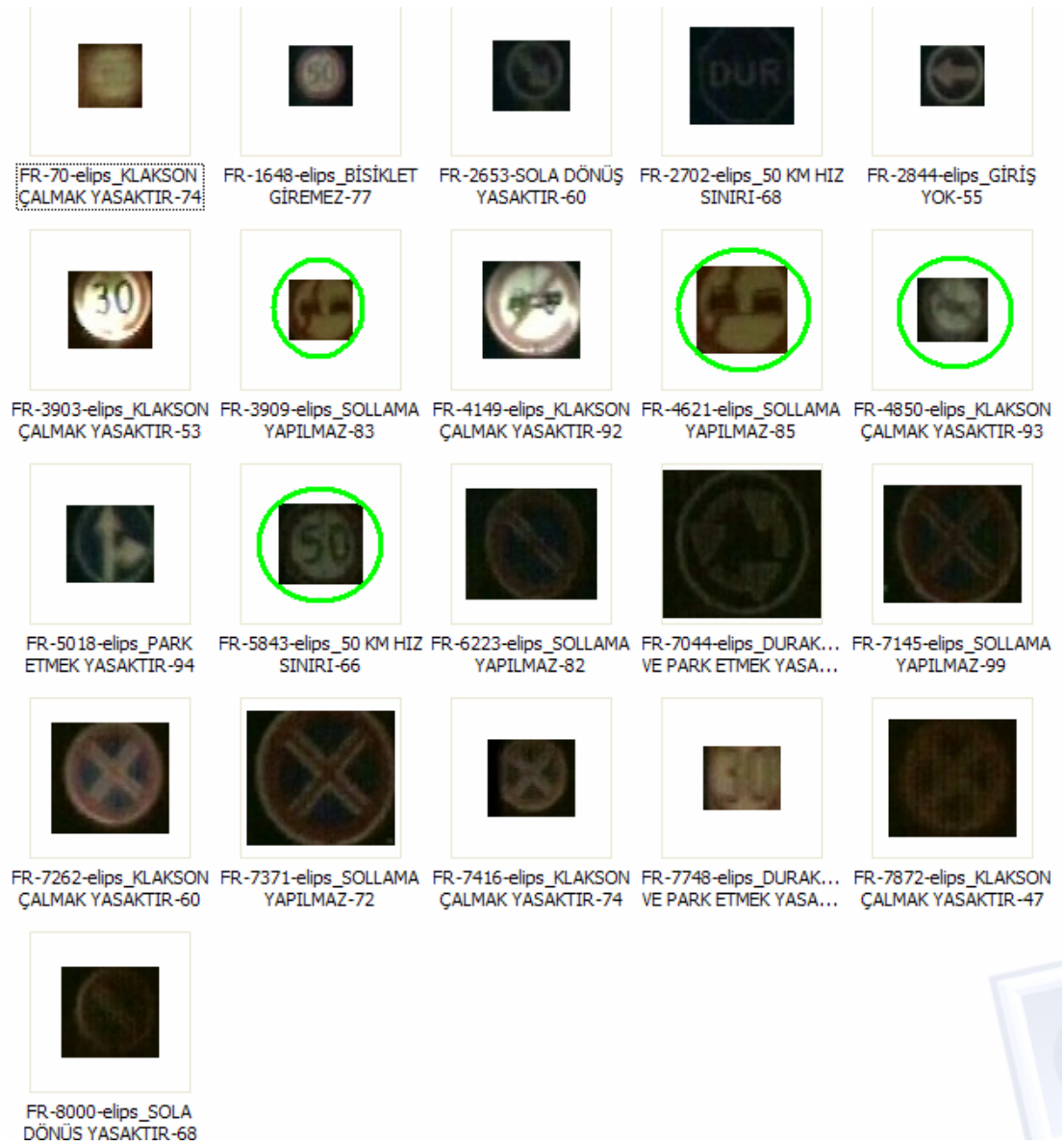
Figure 5.31: Detected and recognized circular signs for Parameter Set-2 and Threshold Set-1 (10 levels) for Table 5.22
