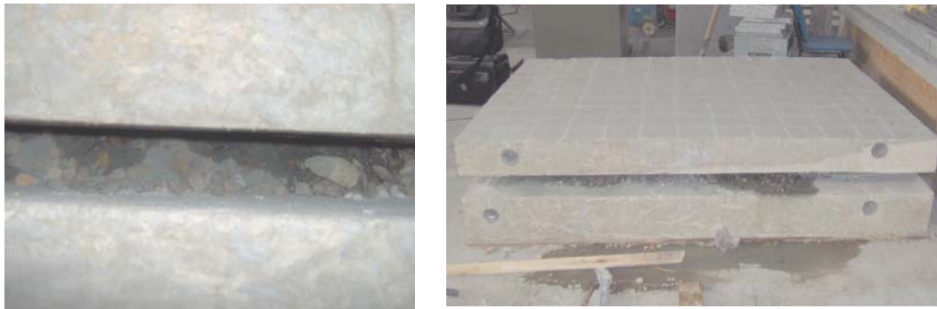
Figure 4.27 The state of the two slabs and the aggregate layer in between before testing
