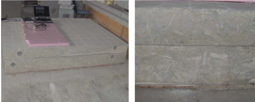
Figure 4.23 Two slabs placed on top of each other for further testing
