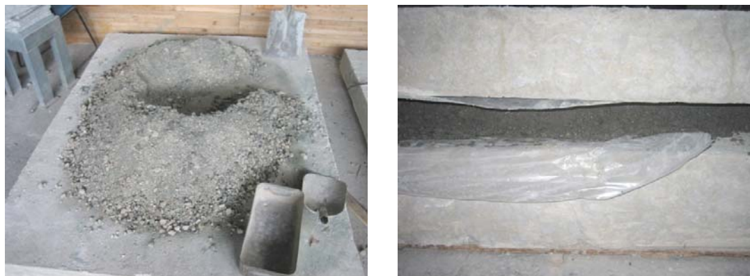
Figure 4.30 Aggregates were mixed with cement in order to produce a lean concrete in between the two slabs
